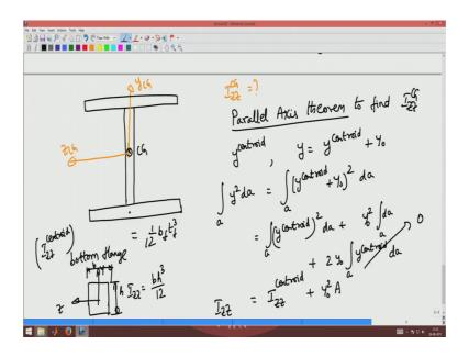
Now, the center of the cross section is this that is the C G and hence your axis would be this will be y and z axis that be a y and z axis about the C G. Now I am interested in finding I z z moment of inertia I z z about the center of cross section is what I have to find. Here what we you make use of is was called as the parallel axis theorem to find the moment of inertia. Here we are going to use parallel axis theorem to find I z z about the centroidal axis ok.
