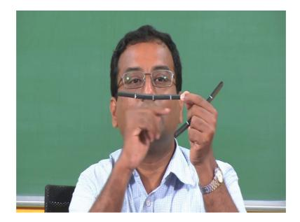
I have this 2 rubber blocks which are not connected to each other. Now, let me say I bend it by applying a non-uniform load, I am bending it by applying a non-uniform load, see what happens at the edges? Then see what happens at the edges? The edges are not flat the plane sections are not remaining plane, there is a shift in the white line and you can see that at this edge there is a zig zag nature of the plane. There the plane is not remaining smooth.
