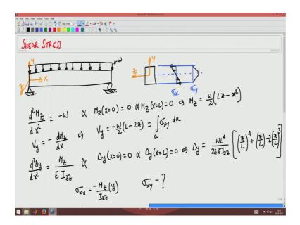
We solve the governing equation d square MZ by dX square equal to minus W with the boundary condition that the moment at the hinged end and the roller end has to be 0 to get the bending moment as W by 2 into LX minus X square.
