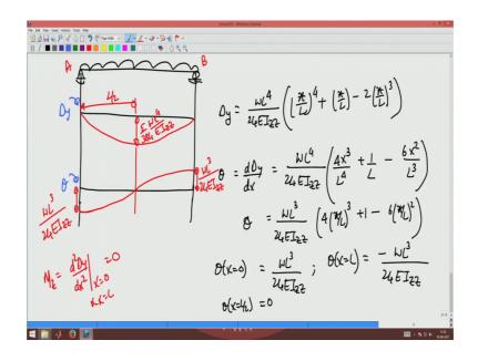
Subject to a u d L we found that delta y is given by W L power 4 by 24 E times I z z into x by L whole power 4 plus x by L minus 2 times x by L, the whole cube. So, it is a 4 third of polynomial and it is deform shape would look something like this; where the maximum bending moment will be 5 by 384 W L power 4 by E times I z z occurring at a distance of L by 2 and that is the location where the slope will go to 0 also.
