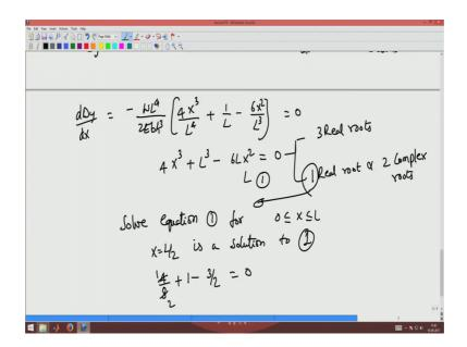
So, d delta y by d x would be minus W L power 4 by 2 E b h cube; the 4 x cube by L power 4 plus 1 by L minus 6 x by L cube, this has to be equal to 0 which means I get a cubic equation here, x cube 4 plus L cube minus 6 L into x equal to 0.
