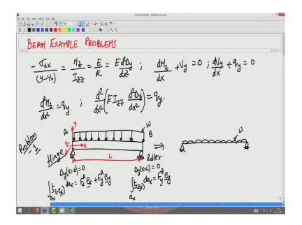
The equation we derived was minus sigma axis by y minus y naught equal to M z by I z z equal to E by R to E d square delta y by d x square, where R is the radius of curvature and then we also saw in the last but previous lecture that d M z by d x plus V y has to be 0, d V y plus by d x plus q y has to be 0.
