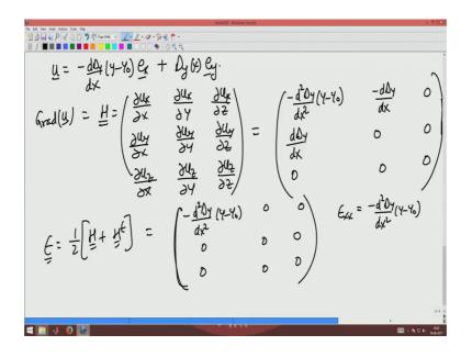
Now, I want to compute gradient of few. So, that I can compute the strain, gradient of u is H which is given by dou x by dou x, if you recollect we saw this 1 we are looking at strains dou x by dou y; dou x by dou z; dou u y by dou x; dou u y by dou y; dou u y by dou z; dou u z by dou z; dou u z by dou z, this for the assume displacement filed would be minus d square delta y by d x square into y minus y naught minus d delta y by d x 0; d delta y by d x 0, 0, 0, 0, 0 ok.
