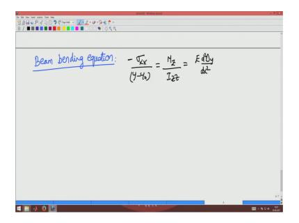
So, combining these 2 equations you get the beam bending equation, which is sigma x x by y minus y naught equal to M z by I z z; E into d x square. So, we have the beam bending equation given by this equation in here.
