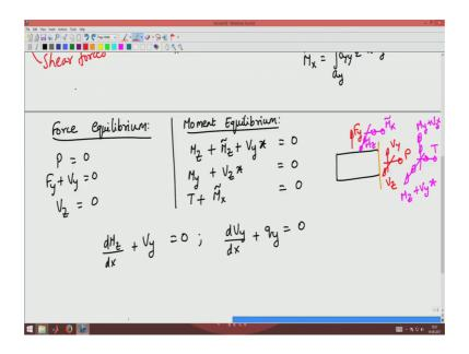
Now, we wrote so the net force and the net moment that is acting on a cut surface of the beam is given here, P acting along the axial direction, V y acting like this, V z acting like this F acting like this, F y acting like this and M z moment acting like this, M x moment acting like this and then M x tilde moment acting along on this phase causing it to twist
