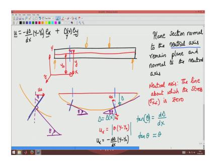
I am going to represent the beam using a 1 dimensional representation that is I am going to represent the central axis of the beam alone. That is, if this is a central axis of the beam, I am going to represent this beam using the central axis alone. The central axis due to the application of a load, some load acting like this, some load acting like this, would deform some load acting like this, would deform into some curved shape like that.
