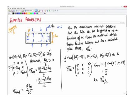
First problem that we are going to look at is a thin walled pressure vessel pressurize from inside subjected to an external pressure P e which is alpha times the internal pressure P i. This pressure vessel has a diameter of 2 times R m, or R m is the radius of this vessel. And t is the thickness of the vessel, ok.
