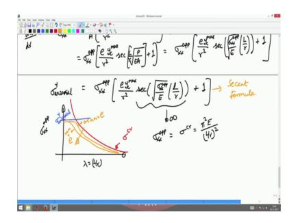
Now, so, I have this to be limited to sigma y uniaxial since the state of stress is uniaxial and if the yield stress is sigma y uniaxial this will be limited to sigma y uniaxial, this will be sigma xx apparent into e yc max divided by r square into secant square root of sigma xx apparent by E into L by r plus 1 ok.
