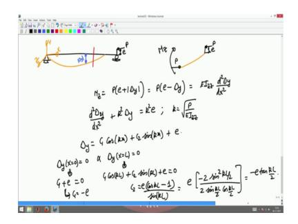
I will go back to a simply supported beam, simply supported column width and eccentrically applied load P I add this eccentricity e coming in there. E might be a small value, but it has an eccentricity e.
