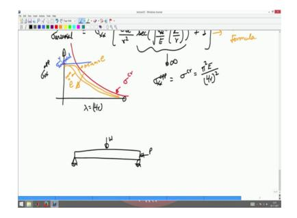
Wherein you are simply supported beam whereas, simply supported beam wherein you can say I applied a lateral load w like this ok. Then also you can redo the analysis get the critical load for this beam to be the same as pi square e by lambda square and you can show that all that what we did now also volts I will would not be doing that in this course.
