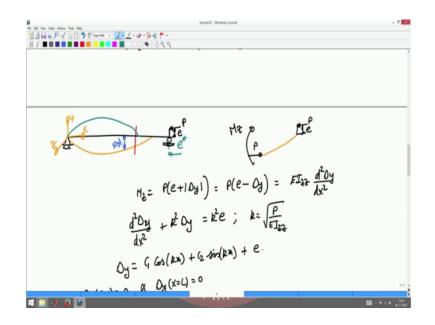
So, if I add a load acting with which is a eccentrically displace upwards, then this column will deform only down. On the other hand if I add this load eccentric downwards this column would deform something like that ok.
