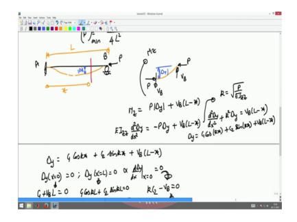
So, essentially you will find that the statement that, if there are no vertical forces acting on the beam there would not be any vertical reaction first (Refer Time: 00:24) is not always true. It depends upon whether the beam is statically determinate or indeterminate the indeterminate system there can be a vertical reaction first (Refer Time: 00:34) even though there is no vertical forces acting on a beam ok. So, that is what I want to emphasize here.
