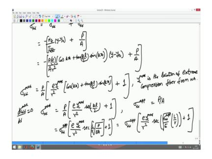
If I were to find the sigma axis max by dx equal to 0 to find the maximum location along the z direction plug in be L by 2 and ends sigma xx max both in x and y would be P by A e yc max by r square into same expression as before this will be secant kl by 2 kl by 2 plus one.
