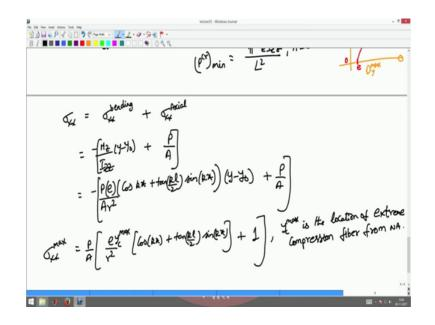
So, we found delta y max, we found delta y I have to find the stress now the stress is given by sigma xx is due to bending plus sigma xx due to the axial force that is applied bending stress is given by minus Mz by Izz into y minus y naught from the bending equation and this is given by P by area of cross section A.
