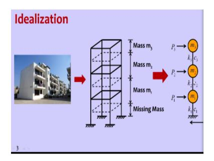
Now if you look at a building a complex system that can be idealized as number of degrees of freedom as many, as number of floors. So in this example you can see a building which is of three floors, so we are converting that into three lumped mass systems. So 3 degrees of freedom system, so this is idealization.
