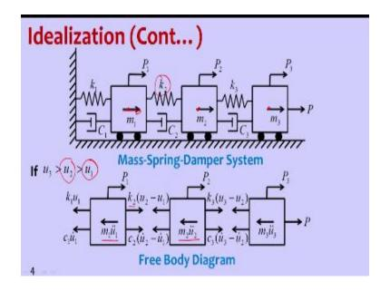
So this is mass spring damper system so the same thing we are representing in mass spring damper system, so mass 1 is represented here damping 1 and stiffness 1, mass 2 is represented here damping 2 and stiffness 2 mass 3 damping 3 stiffness 3 so these are relative properties between 2 floors.
