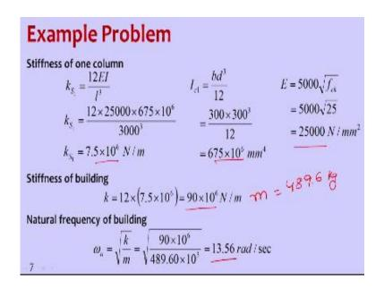
So as we have already discussed in week 7 tutorial mass of each floor is calculated and mass of first and second floors this one 76.6 9 into 10 to the power of 3 kg and mass of the top floor alone is around 130 6.22 into 10 to the power of6 kg so all put together what we are trying to do is we are calculating the mass of total structure wherever even though it is a three-story structure even though this can be lumped as a three-story structure as a multi degree of freedom system.
