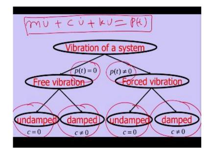
Forced vibration and the another case is un damped free vibration damped free vibration and then un damped forced vibration damped forced vibration so these are the four cases so which will discuss in subsequent modules.
