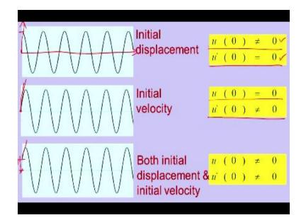
Now initial displacement, initial velocity or both so if we give initial displacement here and as you can see in the horizontal axis this is time scale and when we are giving a time T=0. Some initial displacement so which we are calling it as initial displacement. Here U is 0 U at time T=0  $\neq$  0. So that means some non zero displacement is given and U. Which is velocity at the initial time.
