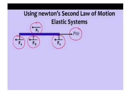
Now we derive dynamic equilibrium equation using Newton's second law. So if we write say a cut the system and write free body diagram this external force is applied here and then inertia of force is opposing the motion and then this is stiffness force, this is stiffness force but which is coming from k/2 and this is damping force.
