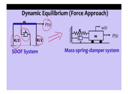
So this is like single degree of freedom system mass is the there springs are there and then damping is there and external force is applied on the system now if we idealized these system as mass is spring damper system so mass means damper system means say if I am vibrating.
