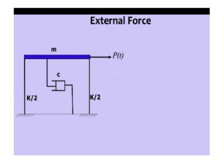
So let's look at how the external force is applied on the structure as you can see the system are the single degree of freedom system can
