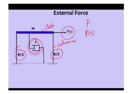
Damping as a dash spot, damping as dash spot. So mass of the structure and then resistance comes by the column which we are representing as stiffness and damping reduces the energy in vibration. In this P is the external force which is being applied now this P as an external force which this is not a static force. A static force is always constant were as dynamic force always changes its value according to time.
