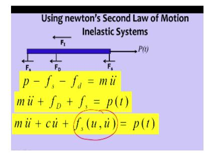
So if the same thing if we write in elastic systems which will become like this here resistance resisting force is not only function of displacement but also it is a function of velocity.
