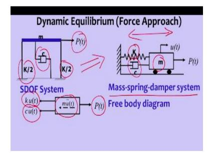
So in this one if I'm idealizing it as mass spring damper system and give initial displacement to this one so this will set to and fro motion now for dynamic equilibrium equation. So what I am doing is I am drawing a free body diagram here so this free body diagram is mass that inertia force because the mass is in the direction opposite to the application of the force that you can see in terms of MÜ.
