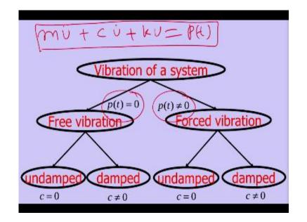
This is free vibration and forced vibration means like when externally applied force is there which is dynamic in nature so that is D'Alembert's principle thank you .
