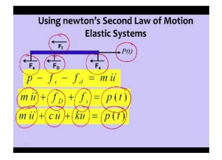
So the same thing can be written like inertia force, damping force stiffness force which is elastic resisting force applied force.
