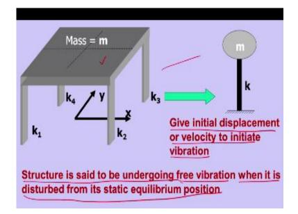
So give an initial condition that is either velocity or displacement to initiate vibration. And the structure is said to undergo free vibration when it is disturbed from its static equilibrium positions so this idealized system can be represented by mass and stiffness mass and spring system.
