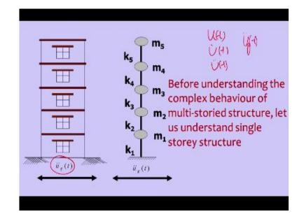
The U double dot G so we, call U as displacement U. which is a deviatory of displacement as velocity and U.. Is a acceleration of the structure and when we use suffix G we call that as acceleration of the ground. So this building is subjected to earth quake ground shaking so a multi-story building. So this multi-storied building can be idealized as many degrees of freedom.
