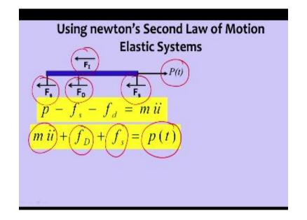
Then MÜ then damping force then stiffness force which is equal to the external force.
