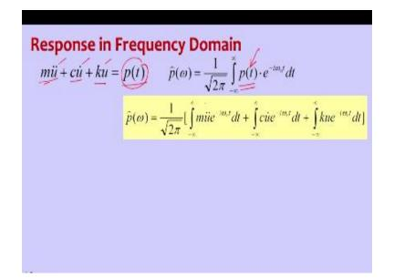
So this is equation of motion so  $M\ddot{U}+CU \text{ dot} + KU=P(t)$ . so the dynamic equilibrium equation so first term is inertia force second term is damping force and third term is stiffness force and all put together is equal to the external force. So we need to convert this force this into frequency domain so by using that Fourier transformation payer so this P(t) put at the time function and then convert that into frequency domain so it something like that.
