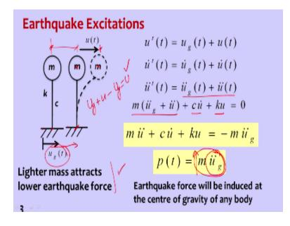
First let us discuss earthquake excitation. So earthquake excitation is let us assume that this is a structure, earthquake excitation means force is acting that is excitation ground is exciting. So ground is vibrating like this. So when ground is vibrating so you can see that because of this ground, ground motion, so ground is moving and structure is vibrating here okay.
