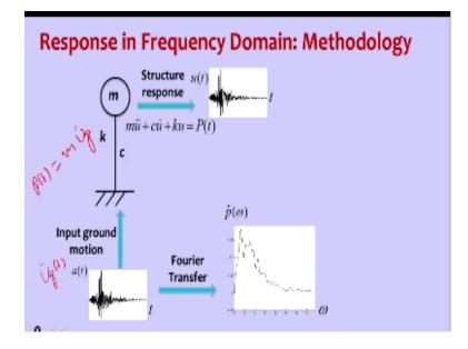
Now let us discuss response of structure in frequency doming so the methodology is as follows so this is the structure which is have been mass damping and stiffness so three parameters mass of the structure damping of the structure and stiffness of the structure if we give input ground motion to this structure then we get response of the structure in time doming so how we get that is mu double dot + cu dot + ku is = p(t).
