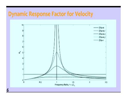
So the graph if we plot this ne the graph what we will get is like this okay again in this one you can see when damping is not there this value is goes to infinity and with the presence of damping that peak amplitude drastically reduces.
