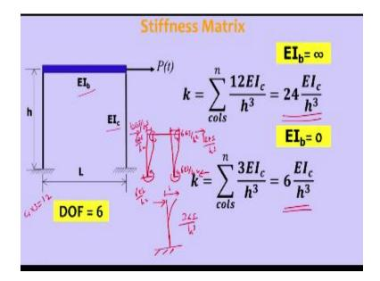
Now let us develop stiffness matrix for a given structure given flame frame structure, in this you can see like being is having length L and height of the column is H  $EI_C$  is given this is fractural visibility of column and fidelity edge of column one and column 2 both are same and flexural visibility of being  $EI_b$  is given and a force is applied at this level at the roof level so in this one the degrees of freedom are 6 so how does degrees of freedom are 6?
