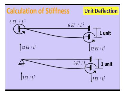
Now when it comes to one unit deflection given at one end of the member, as you can see here like a member where far end is fixed and the near end is rigid, so to that we are giving one unit displacement because of this one unit displacement to maintain zero angle here a rotation have to be applied so that rotation value is  $6EI/L^2$  and the same rotation need to be applied on the other end also  $6EI/L^2$ .
