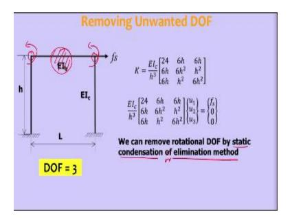
The degrees of freedom is here degree of freedom is here rotation is here rotation is here and translation so translation means entire mass is concentrated this one so that means translational degree of freedom that is degree of freedom one has mass associated with it but degree of freedom 2 has 0 mass and degree of freedom 3 has 0 mass so in this situation how do we remove unwanted degrees of freedom from the equation.
