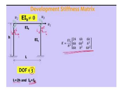
By using l= 2h and moment of in h of column is = moment of in h of  $I_b$  so up open simplification the total 3/3 matrix is this, now after finding out after generating the stiffness matrix if there are no forces associated with the degrees of freedom available it is something like this you can see in this one. (Refer Slide Time: 22:25)
