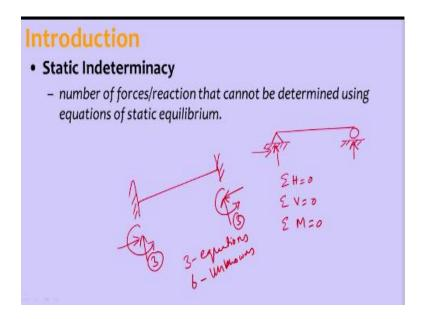
So static indeterminacy means number of forces or reactions that cannot be determined using the equations of static equilibrium. So for example, o if I take a simply supported beam here hinge is there and a roller is there. So roller is vertical reaction comes here and here vertical reaction as well as horizontal reaction comes. So three unknown reactions are there, three unknown reactions and we have three equations of equilibrium  $\Sigma H=0$ ,  $\Sigma V=0$ ,  $\Sigma M=0$ .
