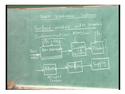
After this coagulation flocculation we will be having a secondary sedimentation tank were all the flocs will be separated. After this coagulation flocculation we have to go for filtration; either slow zone filter or rapid zone filter and here we can add even chlorine to prevent the biological growth.
