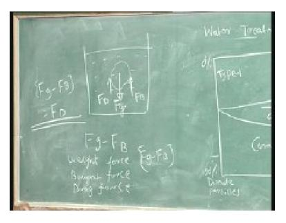
Another force acting on the body is the drag force  $F_D$  so the three different forces acting on the body are the force due to weight force, buoyant force and drag force. Thus, by considering these three forces we can find out the settling velocity of the particle.
