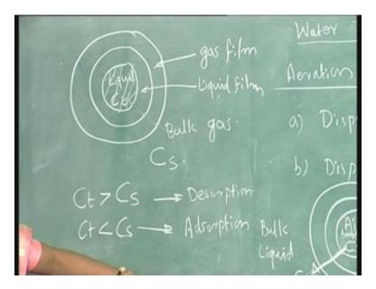
This is the principle of aeration. In case of water treatment systems in aeration most of the time what we do is dispersing water into air this is what we usually go for. So we will see what are the different systems adopted for the dispersion of water into air.
