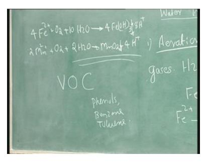
Similarly manganese oxide also can be removed. But manganese oxide precipitation is a very slow process at low pH, means the pH less than 9 the manganese oxide precipitation is low. So if you want to increase the reaction rate what you have to do is you have to increase the pH of the system. This is what is happening in aeration.
