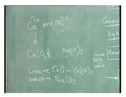
Here what we are doing is we are adding lime and soda so if you add lime and soda the hardness is **coarse** because of divalent cations especially the presence of calcium and magnesium causes hardness which we have discussed in the last class. How can we remove this hardness? We can precipitate out this calcium and magnesium.
