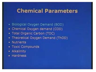
For example, we were discussing about the BOD test we want to conduct for industrial wastewater where there is no biological matter or microorganisms present. At that case we have to add some external seed to the system then only we will have microorganisms to do the work. Then we were discussing about how to find out the biodegradable organic matter concentration and how the BOD or the biodegradation rate depends upon.
