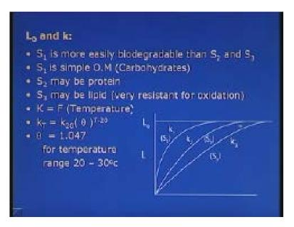
This is the L 0 that means the maximum value we are going to get and this is we have plotted with respect to L and time. So we can see that this is the profile for k 1 and this is for k 2 and this
