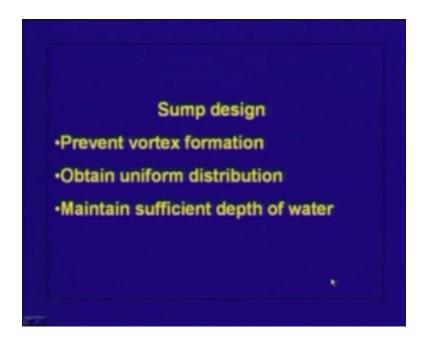
We also have to maintain sufficient depth of water in the sump to prevent air entry. A typical design for a pump sump is like this
