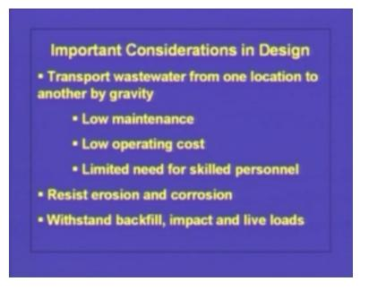
The other one is while designing we design the system such that the sewers can resist erosion and corrosion.
