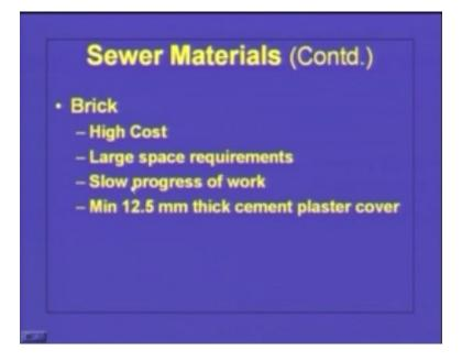
One important consideration is we should have a minimum of 12.5 mm thick cement plaster cover when we are going for brick as a sewer material because if you don't have this sewer plaster cover then the sewer line could be leaking profusely.
