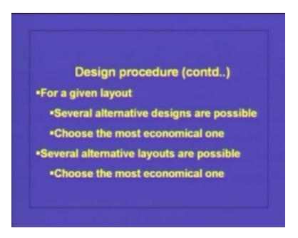
The cost is based on the diameter of the sewer line, the depth of the trenching and what could be the operating costs if some pumps are provided and what could be the maintenance costs depending upon the depth of burial and so on. We work out the total cost the capital cost plus the operating cost plus the maintenance cost. We choose that alternative which gives the least cost or the most economical one.
