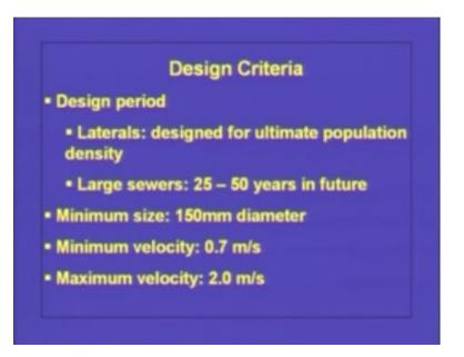
Typically laterals are designed for ultimate population density in a particular area whereas a large sewer is designed for 25 - 50 in future. The minimum size is another important criteria. We should not use any sewer line which has a diameter less than 150mm because this may lead to the problems in the maintenance. So the minimum size for a sewer line is 150mm. As I already talked about, why we should maintain a minimum velocity in a sewer line?
