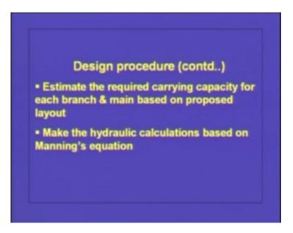
For example, if we consider this particular sewer line, this particular sewer line should carry all the wastewater that is coming from here that is coming from this lateral, that is coming from this lateral and that is coming from this lateral (Refer Slide Time: 28:28) combined the discharge from 1 2 3 4 these four laterals is appearing in this particular line so it should be designed for that whereas this particular line is designed only for the
