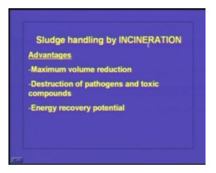
At high temperature whatever is the organic matter present in the system will be getting oxidized and converted to carbon dioxide and water if the process or the system is working with 100% efficiency. Here the destruction of pathogens and toxic compounds are almost cent percent. Moreover, because when we incinerate the solid waste lot of heat energy will be produced and that energy we can recover it and reuse it so energy recovery potential is also there for this process.
