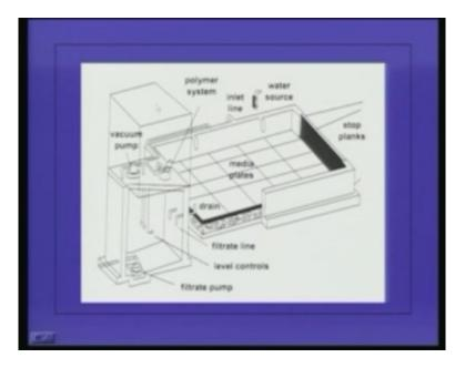
This is the vacuum pump and the filtrate is coming here and filtrate is pumping back. This is a very costly affair so most of the time we are not going for this type of sludge drying bed. Another method of water removal is reed beds.
