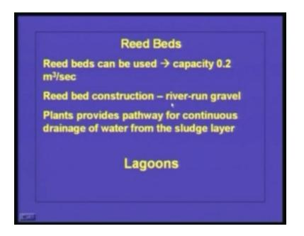
Reed beds can be used and the capacity of the reed beds is around 0.02 meter cube per second and it is constructed using river-run gravel.
