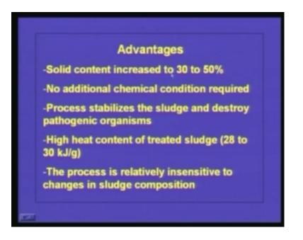
As the heat treatment because it reduces the water content it improves the heat content of the treated sludge. Usually the heat content will be increased up to 28 to 30 kilo joules per gram and this process is relatively insensitive to the changes in sludge composition. We know that the sources of sludge are different.
