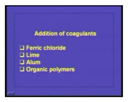
So the most commonly used chemicals for this conditioning are ferric chloride, lime, alum and organic polymers. In this if you add organic polymers it is not going to increase the solid contents of the sludge but if you add ferric chloride lime or alum the organic content or the solid content of the sludge can be increased.
