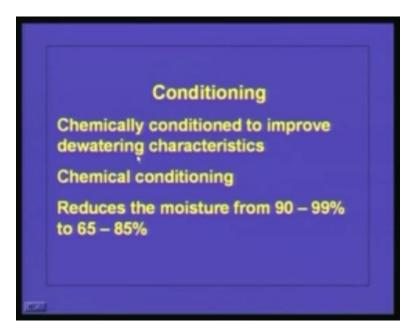
Conditioning is basically used to improve the dewatering characteristics of the sludge. What we are doing here is after the stabilization of the sludge in some cases the stabilized
