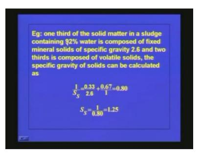
One third of the solid matter in a sludge containing 92% water is composed of fixed mineral solids of specific gravity 2.6 and two thirds is composed of volatile solids, the specific gravity of solids can be calculated as given below.
