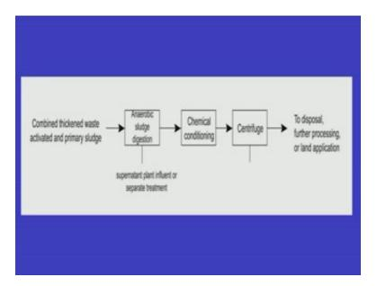
This is the third alternative the combined waste from the activated and primary sedimentation tank is coming and again we are going for anaerobic digestion and the plant effluent whatever is coming is going for further treatment.
