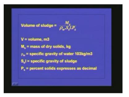
We have seen how to calculate the specific gravity of the solids as well as the specific gravity of the sludge. And if you know the solid concentration as weight then we know how to calculate the volume of the sludge. All these information are available and we know that from each unit what is the nature of the sludge that is coming and what is the amount of the sludge coming out and what is the solid concentration that is coming out, we have seen all those in detail.
