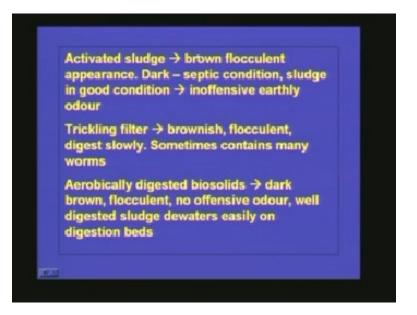
Sludge: Usually the color of the sludge will be brown and it is flocculent in nature. And if the sludge becomes septic then it will become dark. And if the sludge is in good condition it doesn't have any smell or it is inoffensive and it will be having an earthy odor. But if it is dark and septic it will be generating offensive odor. This is the nature of activated sludge and mostly it is organic matter.
