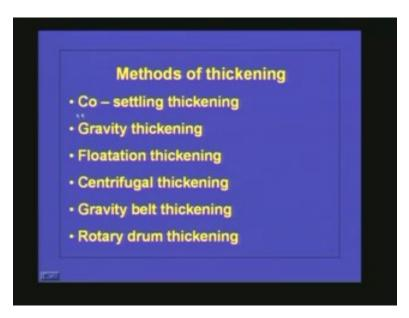
In co-settling we will be having various clarifiers and the sludge from the clarifiers will be coming to the thickener. Similarly the overflow from the clarifiers also will be coming to the thickener. So because of this one a proper thickening will be taking place in the thickening tank and it will be considerably reducing the sludge volume.
