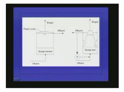
This is another type of reactor so there is no separate GLSS that means Gas Liquid Solid Separator. this is the plastic cover (Refer Slide Time: 26:05) the influent is coming sludge blanket it is here, the velocity is adjusted in such a way that by the time the water reaches here or the treated water reaches here all the biomass whatever is present in the system will be coming back to the sludge blanket, by this way the biomass concentration in the system will be increased.
