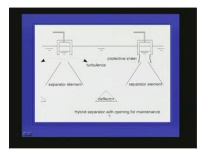
This is a separator with atmospheric pressure because it is exposed to the atmosphere. Here we have easy accessibility and this is a hybrid one and this is a submerged one (Refer Slide Time: 53:12). We will see what all are the advantages of a submerged separator.
