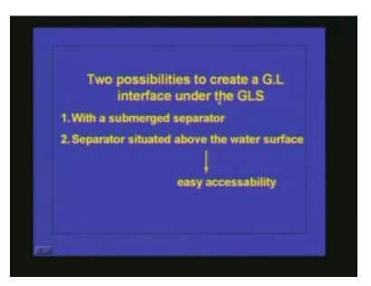
There are two possibilities to create a GL interface. One is with a submerged separator and another one is a separator situated above the water surface. If the separator is situated above the water surface we have easy accessibility. But most of the time we go for submerged separator.
