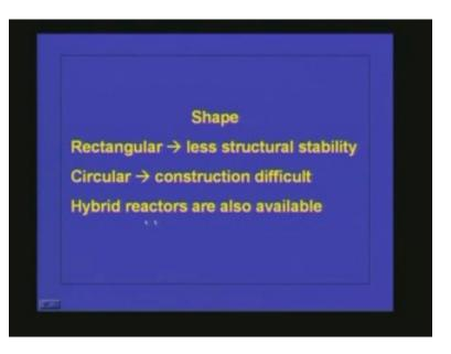
Nowadays people are going for even hybrid reactors. That means the bottom portion is circular or the top portion is rectangular and vice versa the bottom portion is rectangular and the top portion is circular. So these are the geometrical shapes of UASB reactor.
