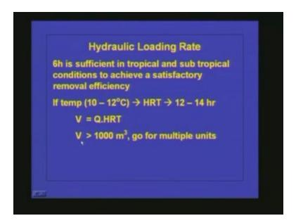
But if the temperature is less then we have to provide a high hydraulic retention time. And if we want to find the volume of the reactor, we know the flow rate of the wastewater Q and if we multiply the flow rate with a hydraulic retention time we will be getting the reactor volume. This is the commonly practiced rule (Refer Slide Time: 46:20), if volume is greater than thousand meter cube go for multiple units and if the volume is less than thousand we can go for a single unit.
