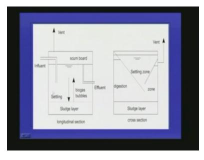
This is the reactor or any closed container and it is not open to the atmosphere only one pipe is there and the influent is coming like this (Refer Slide Time: 3:12) and enough detention time is provided so that all the organic matter in the suspended form will be settling down. Yu will be getting a sludge layer here, the sludge layer will be having so much of organic matter and the oxygen availability is almost nil so the entire system will be under anaerobic condition.
