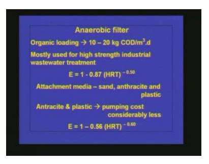
As I have already explained in the anaerobic filter we can go for very high organic loading that means in the range of 10 to 20 kilograms COD per meter cube per day and it is mostly used for high strength industrial wastewater treatment. We can derive the equations for efficiency using kinetic approach. But there are empirical expressions available if you want to find out the efficiency of the system.
