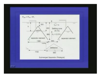
How to design a solid liquid separator?
