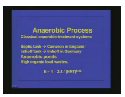
The settling time is so large that means it gives time of 5 to 10 days so during this period whatever suspended solid is present in the wastewater will be settling down and at that time it will not be having any oxygen supply. So what will happen in the sludge settled in the bottom of the tank is it will be under anaerobic conditions. At this condition anaerobic
