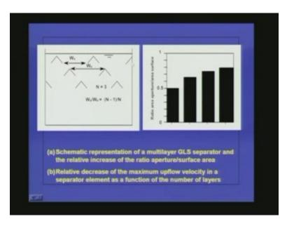
So, instead of providing the GLSS as a single row we can even provide them as different roles so that the efficiency will be much more. So if you want to see the principles of design of a GLSS this one is very very important. This portion we will discuss in detail in the next class because we have to see how the influent arrangement, the effluent arrangement and how to provide the inclination and all other dimensions of a GLSS.
