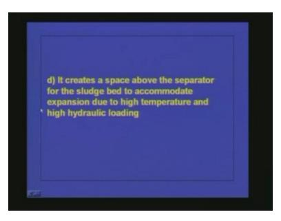
So whatever excess loading comes to the system the reactor will be able to take care of it because it is having a huge area above the solid liquid separator.
