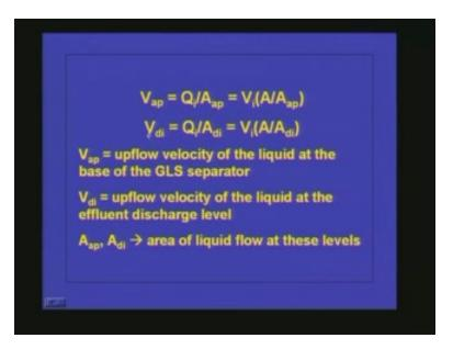
These are the velocities. So if you want to find out the velocities whatever is coming in the aperture and this is the discharge velocity AVp Vap that is nothing but the up flow velocity of the liquid at the base of the GLS separator then we know what is Q and what is the cross sectional area then we can find out that velocity and Vdi which is the up flow velocity of the liquid at the effluent discharge level. That also we can find out if you know the area at the discharge level.
