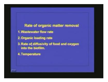
Now we will see how the organic matter is getting removed in the system. The rate of organic matter removal is depending upon the wastewater flow rate and organic loading rate, rate of diffusivity of food and oxygen into the biofilm and the temperature how these parameters are very very important.
