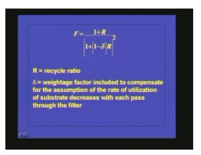
That means kilogram per day without any recycle and V is the volume of the filter in meter cube and F is equal to 1 for no recycle. Hence, if we know the BOD applied per day to the bio filter or bio technique filter and the volume of the filter then we can find out the efficiency of the system.
