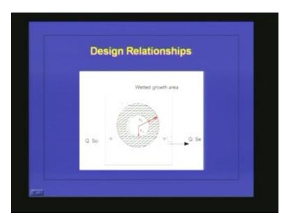
So you have seen that the biomass is growing only in this area and this Q is the flow rate, S0 is the initial BOD, Se is the effluent BOD and this is the biomass growing area. So if you want to make the mass balance how can we do it?
