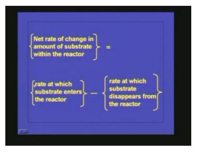
So how can we find out the rate at which the substrate is entering into the system and rate at which the substrate is being removed from the system. The rate at which substrate is entering in the system is nothing but Q into S0 where Q is the flow rate and S0 is the initial BOD of the wastewater and how the substrate is getting removed from the system is equal to ds by dt uA into VA plus ds dt us into Vs plus Q into Se.
