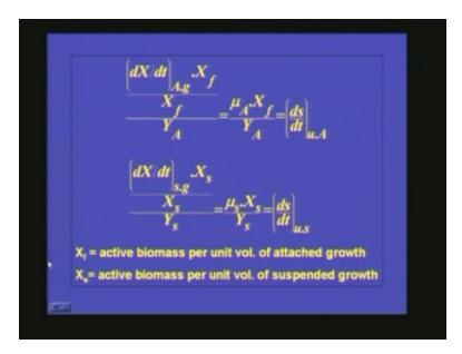
So your final equation will come like this; ds by dt in the total reactor is equal to Q into S0 that is coming in minus Q into Se this is going out minus mu A into  $X_f$  by  $Y_A$  into  $V_A$  – mu s into  $X_s$  by  $Y_s$  into  $V_s$  so this is the substrate utilized by the attached growth system and the substrate utilized by the suspend growth system.
