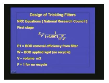
So the most commonly used approach for the design of trickling filter is the NRC equation that means the National Research Council equations. this is the formula; if you want to design the first stage of a trickling filter we can use E1 is equal to the efficiency of the first stage is equal to 1 by 1 plus 0.007 into square root of w by V into F where E1 is the BOD removal efficiency from the filter in the first filter and w is BOD applied.
