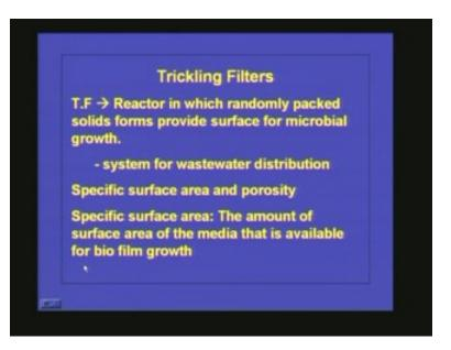
Porosity is the void space available for passage of wastewater and air. So whenever we select a media for the microbial growth porosity as well as specific surface area is very very important.
