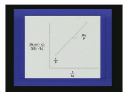
So if you want to find out the P value for a system we can do some large experiments in the law and we can find out this is 1 by Se and this term is equal to 2 into N number of disks into pi into  $r_0$  square minus Re square into Q into S0 minus Se all these terms are
