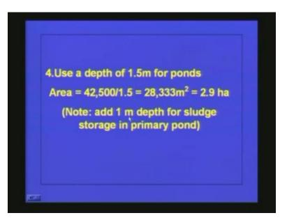
Even though we are providing 1.5 m as the depth we have to give additional 1 m depth because the wastewater whatever is coming to the pond will be having lot of suspended solids so it will be getting accumulated in the system so you should provide in a storage place. That is why apart from the working depth we have to provide 1 m additional depth for the storage of the sludge.
