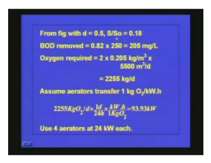
Now we know the k value, we know the theta value so we can find out k theta value. Once you know the theta value and the dispersion coefficient we can refer by to the same figure and get the S by S0 value. That means this will be the efficiency at the time and this value we got from the family of curves is coming as 0.18 which means we are able to achieve only eighty two percentage of removal during summer time.
