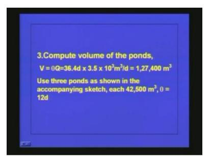
If you go for a series of ponds the efficiency will be higher compared to a single pond because it will be approaching the plug flow regime. So, since we are providing three ponds the detention time of each pond will be around 12 days because three ponds are there and each will be having a volume of 42500. We are getting this value by dividing this 127400 by 3 so the pond system will be like this.
