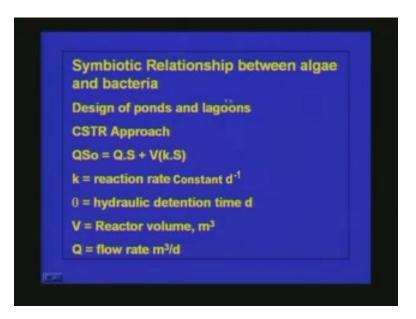
This is the most important thing. If you have more algae in the system definitely the dissolved oxygen concentration in the system will be high. Now we will see how we can design a pond or a lagoon. Either we can go for a CSTR approach or we can go for a plug flow approach so if you want to go for a CSTR approach we can use this equation.
