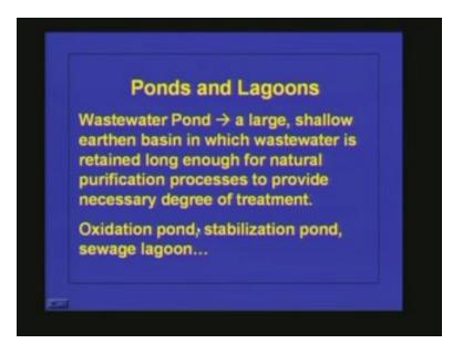
And here the oxygen supply is because of photosynthesis, that is one way how the pond is getting oxygen and another way is the natural replenishment because whatever oxygen present in the wastewater will be consumed by the microorganisms when they utilize the food or it is the biochemical oxygen demand that will be consumed by the microorganisms so naturally the dissolved oxygen concentration in the wastewater will be coming down.
