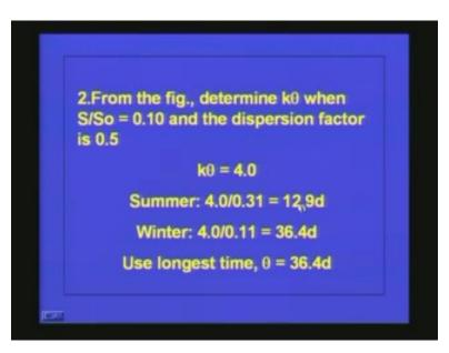
In winter the requirement is 4 by 0.1 because the rate constant is considerably low in winter time so we will be getting a hydraulic retention time of 36.4 day. But whenever we design a system we have to design for the adverse condition so here we have to provide the maximum value of the hydraulic retention time so the hydraulic retention time for the present system should be 36.4 days.
