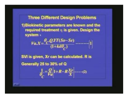
One is the biokinetic parameters are known and the required treatment efficiency is given. We have already found out the biokinetic parameters of the system and efficiency because you know this is the effluent discharge standard we can find out what is the efficiency required. That means you know initial BOD and you know what should be the final BOD so you know what is the treatment efficiency required and how to design the system.
