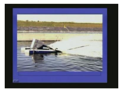
This is a type of brush aerator. It is a surface aerator so it will be aerating the system and it will be giving the horizontal velocity for the flow.
