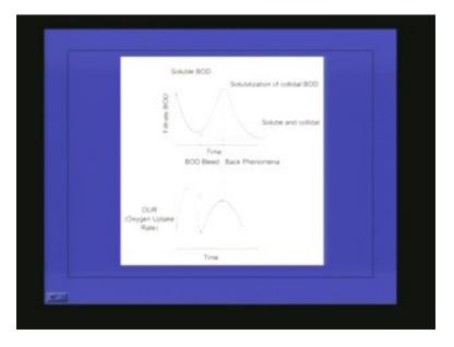
This is the filtrate BOD with respect to time. Initially the filtrate BOD will be very high and the microorganism will start utilizing it so it will be reducing. Only the soluble BOD is there and this will be having a strand like this, it will be going like this (Refer Slide Time: 36:00). But if colloidal particles are there then it will be going like this and mean while the microorganisms will be hydrolyzing the colloidal particles and making them in
