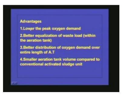
The advantages of this tapered aeration system of stepped system is;
