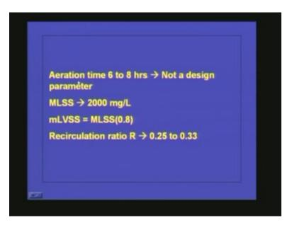
In conventional activated sludge process in aeration tank we give 6 to 8 hours of aeration. And please remember this is not a design parameter. Design parameter is theta<sub>c</sub> and X and Xe we have seen that one on recirculation ratio. But usually this is the time we usually in the aeration tank. In conventional process and MLSS concentration 2000 to
