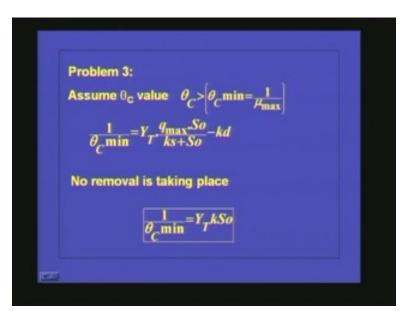
Third problem is theta<sub>C</sub> is not known. So we have the biokinetic parameters. We know that what this theta<sub>C</sub> which is nothing but 1 by mu or 1 by specific growth rate. The mu value is changing for a system but the mu max maximum substrate utilization rate is the constant. If you take one by mu max we will be getting the theta<sub>C</sub> which is required at minimum because as the mu max increases theta<sub>C</sub> value will be decreasing.
