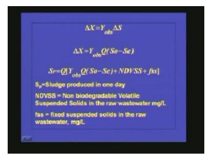
And we know what is the y observed which we can calculate using this formula. We know  $Y_T$  from the biokinetic parameter estimation and kd we know and mu we will be knowing so from that one we will be knowing y observe. This is the total biomass
