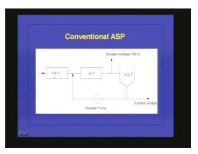
This is the conventional activated sludge process. Primary sedimentation tank, then aeration tank, here we are having the sludge wastage Wc and this is the secondary sedimentation tank and some extra sludge will be there that will be going to the digester and this is the recirculation system and it is coming to the aeration tank.
