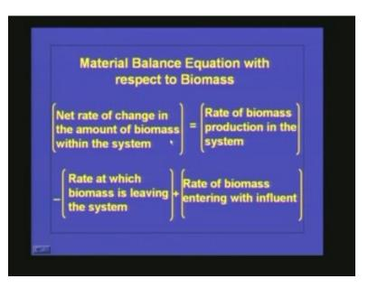
Now we can see how to find out the theta<sub>C</sub> if you know what is the theta<sub>C</sub> we can provide and what is the influent BOD and effluent BOD required. We know what is the treatment required, it should meet the discharge standard. So in terms of BOD it is 30 milligrams per liter. So if you want to find out the volume of the tank how we can go around?
