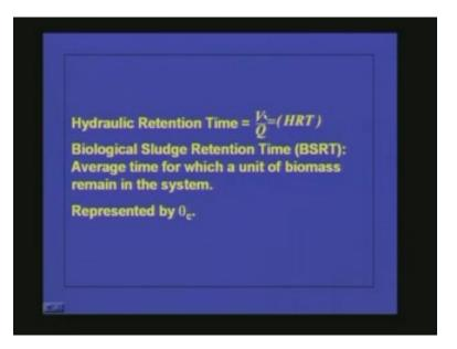
Therefore, v by Q is the hydraulic retention time and another important time is Biological Sludge Retention Time that is BSRT. BSRT is very very important in any biological treatment system which is nothing but biological sludge retention time. The definition is average time for which a unit of biomass remains in the system. The biological retention time is nothing but the total time the biomass staying in the system once the biomass enters the system or is generated in the system.
