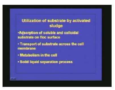
The first one is adsorption of soluble and colloidal substrate on floc surface. Whatever is present in the system has to get adsorbed to the microorganism. Then after the adsorption
