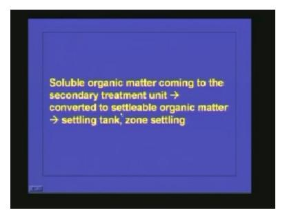
We have already seen that the settling tank the secondary sedimentation tank has to be designed based upon zone settling because the particles are flocculant in nature and it is concentrated suspension. So concentration suspension with flocculant particle is coming under zone settling and towards the bottom of the sedimentation tank the concentration of the particles is so high so they will be experiencing the compression settling.
