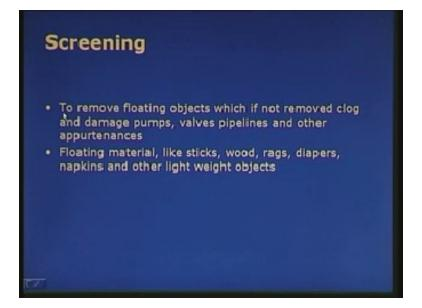
Now let us look at the screening. the objective of the screening is to remove floating objects present in the wastewater which if they are not removed they clog the pumps they damage the pumps, valves, pipelines and other appurtenances that are present in the wastewater collection system. So the wastewater collection system is hampered is damaged because of the floating objects that are present in the wastewater.
