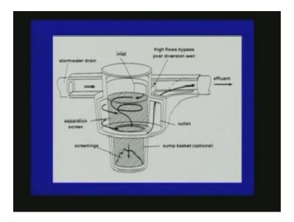
This is another type of screen where the material comes in here, the liquid comes in and flows through this and gets screened. The effluent after screening will go out like this. This (Refer Slide Time: 27:25) is the direction by which it goes, this is the influent and this gets screened and goes out in this effluent and the screenings are collected at the bottom.
