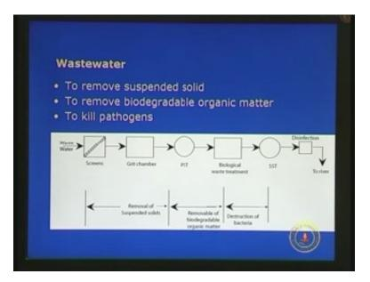
The third one is; the wastewater contains the microorganisms, the pathogens, we have to kill the microorganisms, destruction of microorganisms. For that we again have a treatment system and the treatment system here is called the wastewater treatment system. The wastewater treatment system has several units, there are a number of units in wastewater treatment system.
