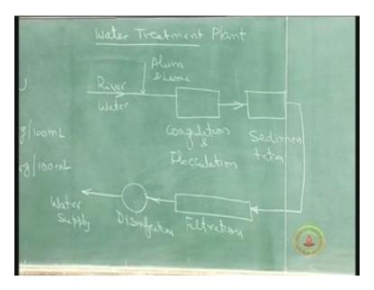
Thus, we have coagulation and flocculation followed by sedimentation and sedimentation is followed by what is called filtration unit and after the filtration unit water moves to a unit called disinfection that is I am trying to kill the microorganisms present in water so this goes to (Refer Slide Time: 5:39) the water supply, this is for water supply.
