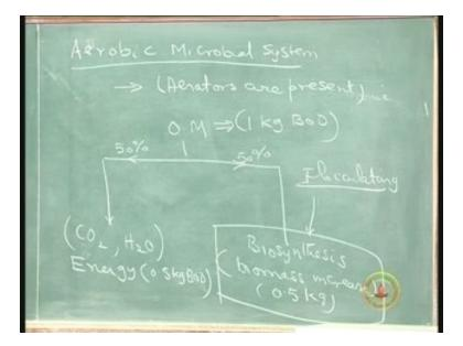
The remaining 50% of BOD that is point five percent of BOD goes into the biomass synthesis. I will get a biomass weight equivalent to 0.5 kg of BOD that is what you are going to get here. So this particular biomass which I am saying here is flocculating in nature. This is flocculating that means it can settle down that is why I have given a secondary sedimentation tank there. You can see a secondary sedimentation tank comes into the picture.
