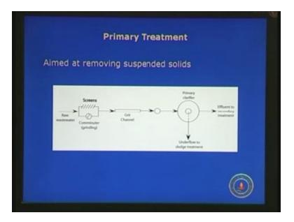
So what I can do is I can divide the wastewater treatment systems into various categories. First one is called primary treatment. I am driving the wastewater treatment system for the convenience of understanding into three segments. One is called the primary treatment. Primary treatment constitutes the following units:
