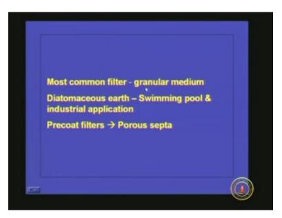
Coming to the practice the most common filter being used in most of the water treatment plants is the granular medium and diatomaceous earth. This is also commonly used in swimming pools and industrial applications and another type of filter is precoat filters. it consists of a porous septa and we add turbid particle or <mark>clay particle</mark> and that will be acting as the filter.
