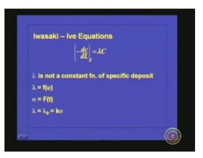
Or we can write like this; C is equal to  $C_0$  into e raised to minus lamda L. So, if you know what is the initial turbidity of the water and if you know what is the length and the filter coefficient we can find out the turbidity that is coming out after the filtration. So this filter coefficient we can find out by conducting the laboratory experiments.
