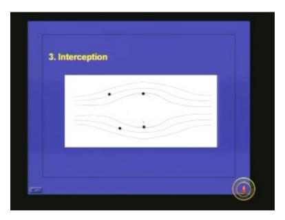
The distance between the filter media and the streamline is less than the diameter of the particle to me removed which is known as interception. So lot of particle can be removed by this mechanism. This is the third transport step. The fourth one is inertial impaction. We know that the turbid particles are having high density compare to the water.
