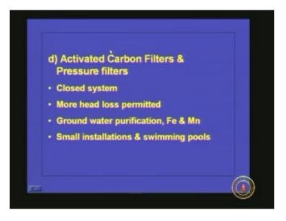
Another one is activated carbon filters and pressure filters. Activated carbon filters are pressure filters usually used in industries so they will be removing turbidity as well as the dissolved solids present in the water because activated carbon as we all know is a very good adsorbent so filtration as well as adsorption will be taking place simultaneously. So depending upon the quality of raw water we can desire which type of filter we have to use and it can remove even dissolved gases.
