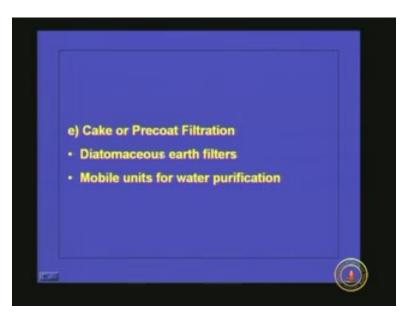
Usually diatomaceous earth filters are used and they are mobile units for water purification. Whenever we have to have a water treatment unit which is mobile at that time we can go for precoat filters as it is very very easy to move from one place to another place.
