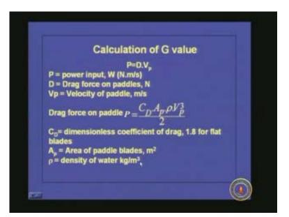
How can we design a flocculator or how can we find the G value?
