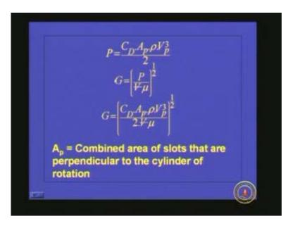
We have already seen that the velocity gradient is nothing but P by V mu raised to half. So G from this one we can calculate; G is CD A p rho V p 3 by 2 V mu whole raised to half. So A p is the combined area of slots that are perpendicular to the cylinder of rotation. That means if you have a flocculator the center shaft will be there and from that one the paddles will be there so we have to take the total area of all the slots that is moving in the water.
