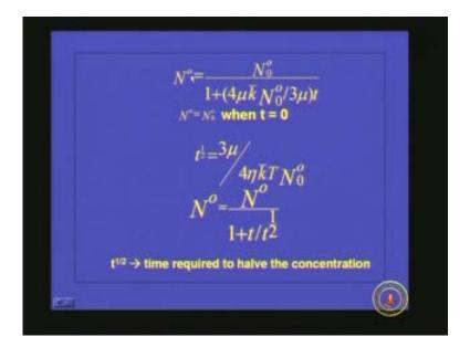
Therefore, the number of particles present in the system at any time can be found out using this formula; N 0 at t equal to 0 divided by 1 plus 4.... If you integrate the earlier equation then you will be getting this value; 1 plus 4 mu k bar into N 0 raised to 0 by 3 mu into t where t is the time. So at any time we can find out what is the number of particles present in the system.
