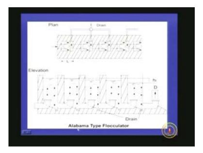
This is another type; Alabama type flocculator. Here what is happening is every chamber is having a separate inlet pipe. We can see here and the coming up like this and since it cannot go
