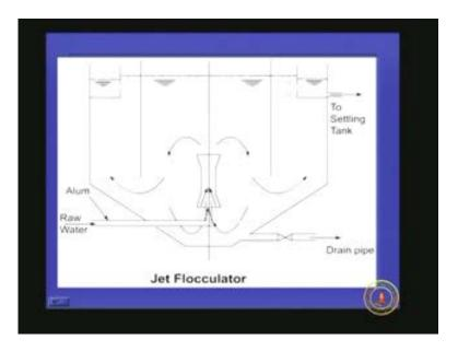
We can see baffles here and as it comes out there will be velocity gradient because the diameter of the tank is increasing with respect to this horizontal distance so the velocity will be varying and the velocity gradient will be created and this is the baffle (Refer Slide Time: 49:14) to avoid the short circuiting otherwise what will happen, everything will be going up and coming out through this outlet so these baffles help to provide more velocity gradient and avoid short circuiting.
