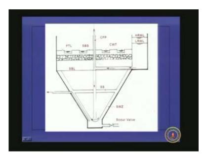
This is the modified type. Here we are providing the pebbles and all so that will be increasing the velocity gradient.
