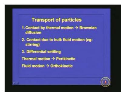
Now we will see what is the mechanism of this flocculation. So it is nothing but the transport of particles. Transport of particles, we have discussed earlier that coagulation and flocculation is the transport of particle and agglomeration of particle. Agglomeration of particle can take place only
