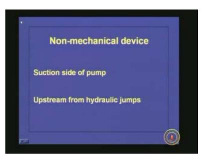
Whatever we have seen now those three units are mechanical units that means they are supplying power by mechanical means or through electricity or whatever and the unit is working but there are many non-mechanical devices which are used for rapid mixing. The advantage of this one is there is no maintenance cost and no energy requirement so it is more preferable but the only thing is if we design this one and construct it we cannot change the system it will be very very difficult.
