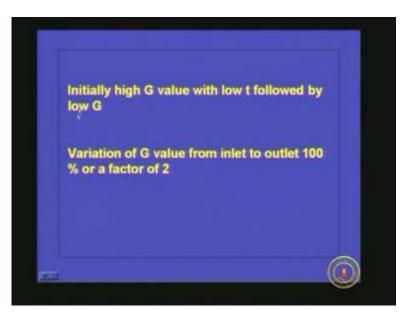
So how can we vary? Initially provide high G value with low t followed by low G value and variation of G value from inlet to outlet, if you want to get the best efficiency it is advisable to provide G value in such a way that the G value is varying 100 percentage from the inlet to outlet. That means the G value in the inlet, if you take the ratio of G value in the inlet to that of outlet if the factor is 2 then your efficiency is maximum.
