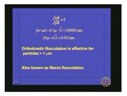
Or in other ways if you want to have a ratio Jok and Jpk that means the removal by Orthokinetic flocculation and Perikinetic flocculation are equal that is what this one represents. Then in
