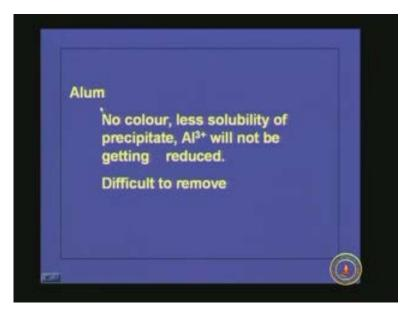
And in water treatment alum is preferred because there is no colour, less solubility of precipitate, and Al 3 plus will not be getting reduced but the disadvantage is aluminum hydroxide flocs are lighter than ferric chloride flocs so the removal is difficult.
