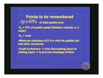
So, whenever we design a flocculator these are the points to be remembered. A p that means the area of cross-section of the paddle should be less than 40 percent of the total paddle area. So, whatever total area of paddle we are providing the cross-sectional area A p should be less than
