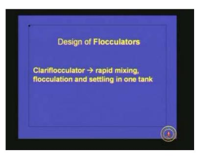
Now we will see how to design a flocculator. In a clariflocculator, clariflocculator is a unit commonly used in water treatment plants so in clariflocculator what is happening is rapid mixing, flocculation and settling is done in one tank so we are providing all the units in a single unit. That is what a clariflocculator is.
