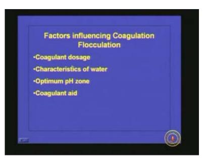
Now we will see what are the factors influencing the coagulation and flocculation. First one is coagulant dosage. Unless we destabilize the particle or unless we provide enough coagulant dose the particles are not going to be removed even whatever best way we design the rapid mixture and slow mixture or flocculating unit and your settler, because unless the particle's destabilization is done properly it is not going to agglomerate. Thus, the coagulant dose is very very important.
