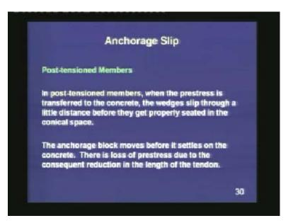
In post-tensioned members, when the prestress is transferred to the concrete, the wedges slip through a little distance before they get properly seated in the conical space. The anchorage block moves before it settles on the concrete. There is a loss of prestress due to the consequent reduction in the length of the tendon.
