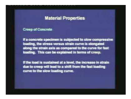
If a concrete specimen is subjected to slow compressive loading, the stress versus strain curve is elongated along the strain axis as compared to the curve for fast loading. This can be also explained in terms of creep. If the load is sustained at a level, then the increase in strain due to creep will lead to a shift from the fast loading curve to the slow loading curve. Let us explain this by a sketch.
