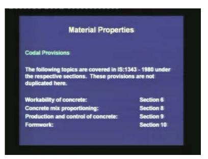
These provisions are not mentioned in detail in this lecture. The provisions are self explanatory, and they can be referred to whenever they are needed. We are just summarising the properties. The code specifies the workability of concrete in Section 6. The concrete mix proportioning is specified in Section 8; the production and control of concrete in Section 9. The specification for formwork is given in Section 10.
