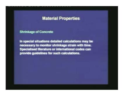
In special situations, detailed calculations may be necessary to monitor shrinkage strain with time. The expression in the code is independent of time; it gives a value of the ultimate shrinkage strain. But if we have to monitor the loss of prestress with time, we may have to estimate the shrinkage strain with time. In that case, specialized literature or international codes can be referred to for guidelines.
