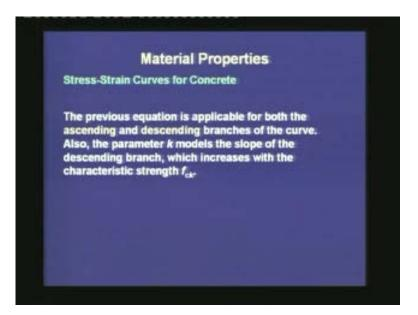
Just to summarize, this previous equation is applicable both for the ascending and the descending branches of the curve. Also, the parameter k models the slope of the descending branch, which increases with the characteristic strength  $f_{ck}$ .
