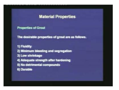
The first desirable property of grout is fluidity, i.e. it can be pumped. Usually the posttensioned members are larger and longer. Hence, if we are pumping the grout from one side it has to reach the other side, and excess amount of grout should flow out to make sure that the full annular space between the tendon and the concrete has been filled.
