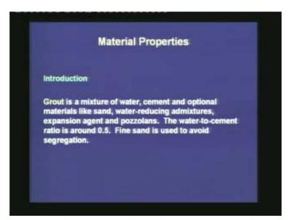
In our previous lectures, we have mentioned that for post-tensioned members it is advisable to grout the tendons, which helps in transferring the stress from the tendons to the concrete over the length of the members. The grout also has an anti corrosive environment for the tendons, and the grout should be strong enough to sustain the load over time.
