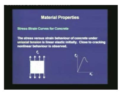
Next, let us move on to the stress-strain curves for concrete under tension. For tension as I said earlier, there are three ways to find out the strength. The first one is a beam under
