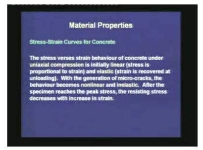
The stress-strain curve under uniaxial compression is initially linear. That means, stress is proportional to strain and in that region it can be considered to be elastic, which means that the strain is recovered if we unload the specimen. But with the generation of microcracks, the behaviour becomes non-linear and inelastic. After the specimen reaches the peak stress the resisting stress decreases with increase in strain. Let me explain this by a sketch. (Refer Slide Time: 03:25)
