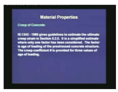
As I mentioned before that the creep strain depends on several factors. The code gives us a very simplified approach to calculate the creep strain, wherein the expression depends on only one factor, and this factor is the age of the concrete at loading (in short, age of loading). The creep coefficient  $\theta$  is provided for three values of age of loading.
