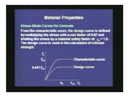
From the characteristic curve, the design curve is defined by multiplying the stress with a size factor of 0.67, and dividing the stress by a material safety factor of  $\gamma_m = 1.5$ . The designs curve is used in the calculation of ultimate strength in a member.
