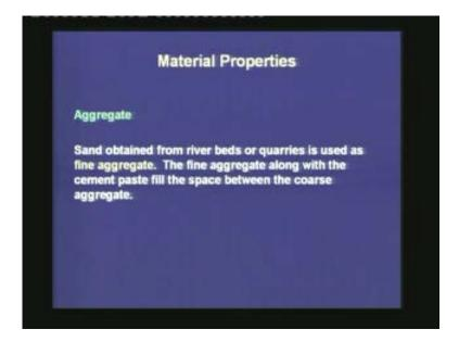
The coarse aggregate is the basic constituent of the concrete, because it covers the maximum volume within the concrete. The next constituent is the fine aggregate. The sand obtained from riverbeds or quarries is used as 'fine aggregate'. The fine aggregate along with the cement paste fill the space between the coarse aggregates.
