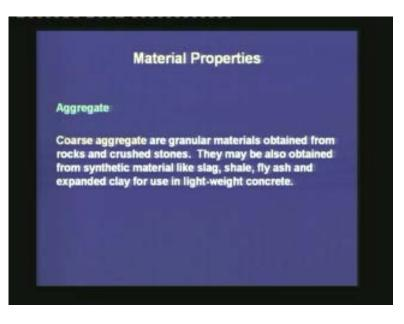
Now, the first constituent, the coarse aggregates are granular materials obtained from rocks and crushed stones. They may also be obtained from synthetic materials like slag, shale, fly ash and expanded clay for use in lightweight concrete.
