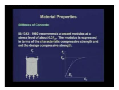
Let me explain these three types of modulus by the stress-strain curve of a cylinder under compression.
