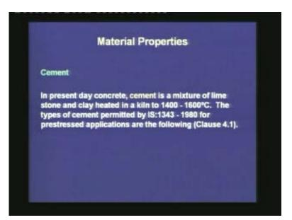
The third constituent of concrete is the cement. In present day concrete, the cement is a mixture of limestone and clay, heated in a kiln to 1400 to 1600°C. The manufacturing of cement is a subject by itself, and it is one of the important inventions in the development of reinforced concrete. The type of cement that is permitted by the code IS: 1343 for prestressed applications are the following. This is given in Clause 4.1.
