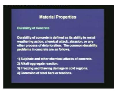
The durability of concrete is defined as its ability to resist weathering action, chemical attack, abrasion or any other process of deterioration. The common durability problems in concrete are as follows: the first one is the sulphate and other chemical attacks of
