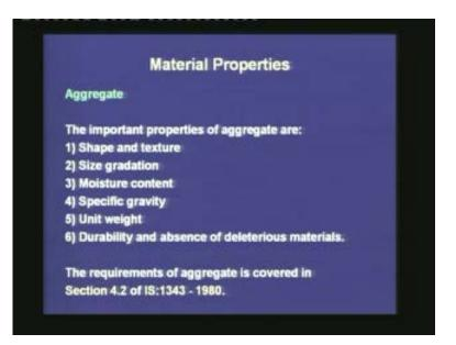
The important properties of aggregates are the shape and texture, size gradation, moisture content, specific gravity, unit weight, durability and absence of deleterious materials. Most of these properties are covered in detail in a course on concrete technology. There are some requirements of aggregate in Section 4.2 of the code IS: 1343.
