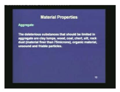
The code says that the coarse aggregate should be free of deleterious substances like clay lumps, wood, coal, chert, silt, rock dust, organic materials, unsound and friable particles. These types of materials reduce the bond between the coarse aggregate and the cement paste. They may also lead to the corrosion of steel, if those deleterious materials are corrosive in nature.
