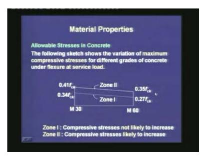
The code specifies maximum compressive stresses for the different grades of concrete, under flexure at service loads. There is no specific allowable stress specified for the intermediate stage, because for this stage, the loading is very case specific. Proper judgment has to be done to analyze a member for the intermediate loading. The code specifies values only for the service loads.
