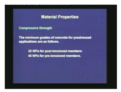
The minimum grades that the code allows for prestressed concrete applications are: 30 MPa for post-tensioned concrete and 40 MPa for pre-tensioned concrete. As we had seen
