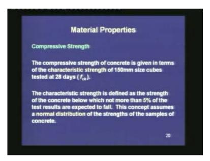
How do we quantify the strength of concrete? We all know that the strength of concrete increases with time. Most of the gain in strength occurs in the first four weeks, and gradually the gain tapers off. The compressive strength of concrete is given in terms of the characteristic strength of 150 mm size cubes tested at 28 days. This strength, which is a standardised measure of the compressive strength of concrete, is called the characteristic strength. This is denoted as  $f_{ck}$ .
