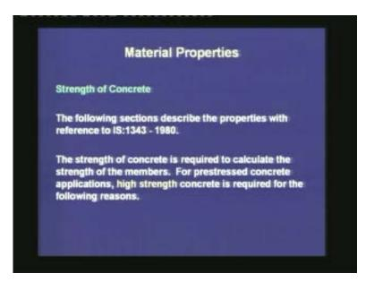
The following sections describe the properties of hardened concrete with reference to IS: 1343. The strength of concrete is required to calculate the strength of the members. For prestressed concrete applications, high strength concrete is required for the following reasons.
