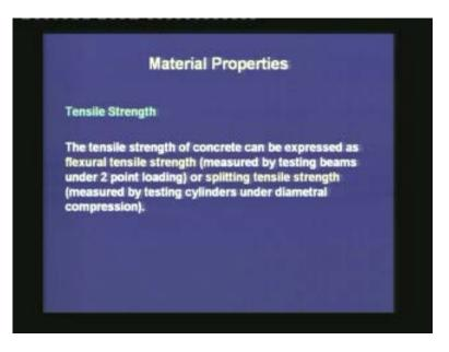
Next, we come to the tensile strength of concrete. The tensile strength of concrete can be expressed by either the flexural tensile strength or the splitting tensile strength. The flexural tensile strength is measured by testing beams under 2-point loading. Sometimes, the 2-point loading is also called as a 4-point loading by considering the reactions. This is a simple test, where the beam is subjected to a uniform moment over a certain region. Let me explain this by a sketch.
