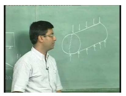
In a splitting tensile strength, a cylinder is laid horizontally and it is applied with a vertical load through its meridian. At a certain time after the load is increased, it splits along the vertical direction and the load corresponding to this splitting gives the splitting tensile strength. Both these tests are covered in detail in the concrete technology course. Hopefully, you should be aware of both these tests.
