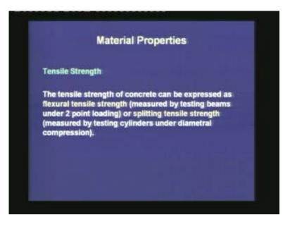
These two tests, the flexural tensile strength and the splitting tensile strength tests are easy to perform. There is a third type of test for calculating the tensile strength of concrete, that is, the 'direct tensile strength test'. This test is more difficult to perform, but still, they are done for research purposes.
