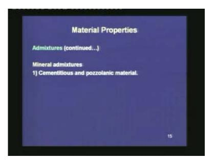
The other type of admixtures is the mineral admixture. The mineral admixtures can be cementitious and pozzolanic material. An example is fly ash. These types of admixtures are used to have some more cementitious material other than the cement, and also to utilise an industrial by-product.
