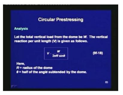
Let the total vertical load from the dome be W, the vertical reaction per unit length which is denoted as V is given as follows: V is equal to W divided by 2 pi times R sin theta. Here, R is the radius of the dome and theta is the half of the angle subtended by the dome.
