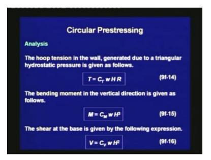
The hoop tension in the wall, generated due to triangular hydrostatic pressure is given as follows: T is equal to  $C_T$  times w times H times R. The bending moment in the vertical direction is given as follows: M is equal to  $C_M$  times w times H cube. The shear at the base is given by the following expression: V is equal  $C_V$  times w times H square.
