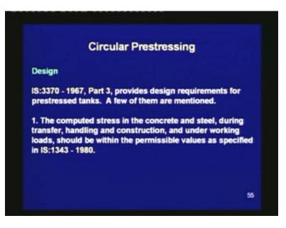
IS: 3370 - 1967, Part 3, provides design requirements for prestressed tanks. A few of them are mentioned. The computed stress in the concrete and steel, during transfer, handling and construction, and under working loads, should be within the permissible values as specified in IS: 1343 – 1980, which is the code for prestressed concrete.
