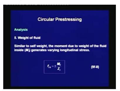
Fifth is the weight of fluid. Similar to self weight, the moment due to weight of the fluid inside, which is denoted as  $M_f$  generates varying longitudinal stress and  $f_{15}$  is equal to plus or minus  $M_f$  divided by  $Z_1$ .
