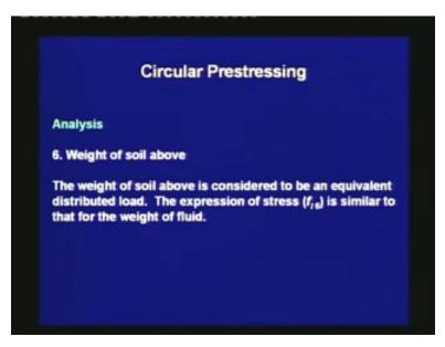
Finally, the weight of the soil above is considered to be an equivalent distributed load. The expression of stress  $f_{16}$  is similar to that for the weight of the fluid.
