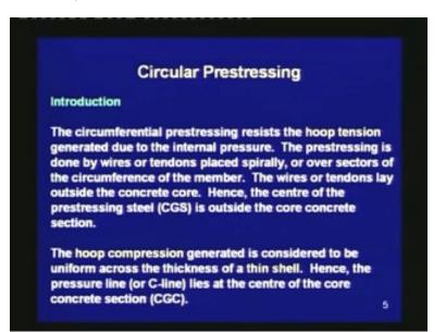
The circumferential prestressing resists the hoop tension generated due to the internal pressure. The prestressing is done by wires or tendons placed spirally or over sectors of the circumference of the member. The wires or tendons lay outside the concrete core. Hence, the centre of the prestressing steel, which we shall denote as CGS, is outside the core concrete section.
