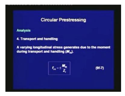
Fourth is transport and handling. A varying longitudinal stress generates due to the moment during transport and handling, which is denoted as  $M_{th}$ .  $M_{th}$  can be determined based on the support points of the pipe. Thus, once the  $M_{th}$  is determined we can find out the stress, which is given as  $f_{14}$  is equal to plus or minus  $M_{th}$  divided by  $Z_1$ .
