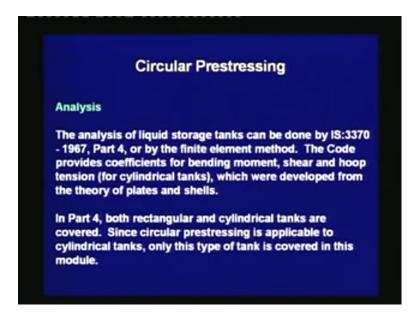
The analysis of liquid storage tank can be done by IS: 3370-1967, Part 4, or by the finite element method. The code provides coefficients for bending moment shear and hoop tension for cylindrical tanks, which were developed from the theory of plates and shells.
