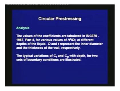
The values of the coefficient are tabulated in IS: 3370-1967, Part 4 for various value of H square divided by Dt, at different depth of the liquid. D and t represent the inner diameter and the thickness of the wall respectively. The typical variations of  $C_T$  and  $C_M$  with depth, for two sets of boundary conditions are illustrated.
