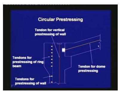
This sketch shows some details of the prestressing tendons. This is at the junction of the dome and the ring beam. The dome is circularly prestressed by tendons, which are first anchored. Then the cylindrical wall is prestressed in the vertical direction; the wall is also prestressed by tendons in the circumferential direction and the ring beam, which is at the base of this dome is also circumferentially prestressed.
