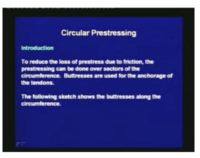
To reduce the loss of prestress due to friction, the prestressing can be done over sectors of the circumference. Buttresses are used for the anchorage of the tendons. The following sketch shows the buttresses along the circumference.
