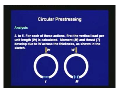
For the other causes, we should understand that due to a vertical load a thrust and a moment is generated in the circumferential direction. For 2 to 5 for each of these actions, first the vertical load per unit length, which is denoted as W, is calculated. The moment M and thrust T develop due to W across the thickness, as shown in the sketch. Thus it is due to the distortion of the pipe that we get the thickness, the thrust and the moment.
