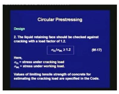
Second, the liquid retaining face should be checked against cracking with a load factor of 1.2. Thus,  $sigma_{CL}$  divided by  $sigma_{WL}$  should be greater than or equal to 1.2, where  $sigma_{CL}$  is the stress under cracking load, and  $sigma_{WL}$  is the stress under working load. Values of limiting tensile strength of concrete for estimating the cracking load are specified in the code.
