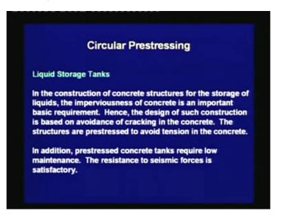
Next, we move on to the liquid storage tanks. In the construction of the concrete structures for the storage of the liquids, the imperviousness of concrete is an important basic requirement. Hence, the design of such construction is based on avoidance of cracking in the concrete. The structures are prestressed to avoid tension in the concrete. In addition, prestressed concrete tanks require low maintenance. The resistance to seismic forces is satisfactory.
