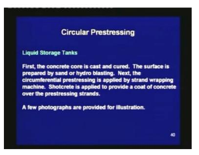
In this type of structures, first the concrete core is cast and cured. The surface is prepared by sand or hydro blasting; this is the outside surface. Next, the circumferential prestressing is applied by strand wrapping machine. Shotcrete is applied to provide a coat of concrete over the prestressing strands. A few photographs are provided for illustration.
