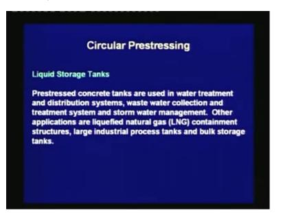
Prestressed concrete tanks are used in water treatment and distribution systems, waste water collection and treatment system and storm water management. Other applications are liquefied natural gas; in short LNG containment structures, large industrial process tanks and bulk storage tanks. Thus, the liquid storage tank has wide application starting from the use of water and waste water to other types of liquid storage which are used in the industrial processes.
