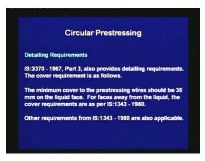
IS: 3370, Part 3 also provides detailing requirements. The cover requirement is as follows.
