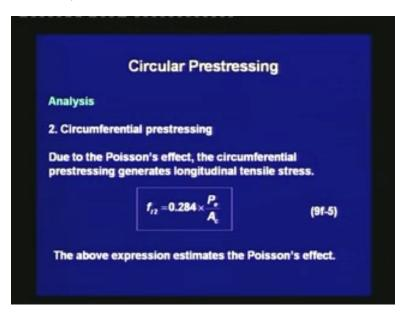
Second is the circumferential prestressing. Due to the Poisson's effect, the circumferential prestressing generates longitudinal tensile stress. It is given as  $f_{12}$  is equal to 0.284 times  $P_e$  divided by  $A_c$ . The above expression estimates the Poisson's effect.
