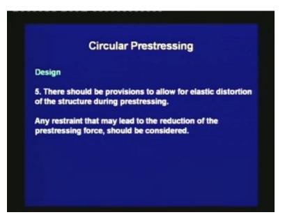
There should be provision to allow for elastic distortion of the structure during prestressing. Any restraint that may lead to the reduction of the prestressing force should be considered. Thus, when the prestressing is done, if there is some restrain, then there can be a drop in the prestressing force and that should be considered in the analysis and design of the prestressed concrete tanks.
