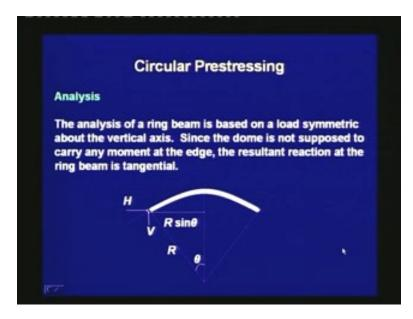
The analysis of a ring beam is based on a load symmetric about the vertical axis. Since the dome is not supposed to carry any moment at the edge, the resultant reaction at the ring beam is tangential. Thus, if we take a free body diagram of the dome, the reaction at the support is tangential. This relates the horizontal thrust on the domes and the vertical reaction on the dome. R is the radius of the dome and theta is half of the angle that is subtended by the dome. (Refer Slide Time 46:38)
