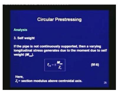
Third due to the self weight, if the pipe is not continuously supported, then a varying longitudinal stress generates due to the moment due to self weight, which we shall denote
