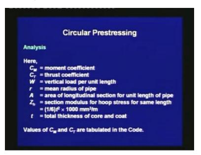
In the previous equation  $C_M$  is the moment coefficient,  $C_T$  is the thrust coefficient, W is the vertical load per unit length, r is the mean radius of pipe, A is area of longitudinal section for unit length of pipe,  $Z_h$  is the section modulus for hoop stress for the same length which is given as 1 by 6 t square times 1000 millimeter cube per meter and t is the total thickness of core and coat. Values of  $C_M$  and  $C_T$  are tabulated in the code.
