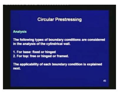
The following types of boundary conditions are considered in the analysis of the cylindrical wall. Number one, for base: fixed or hinged. For top: free or hinged or framed. The applicability of each boundary condition is explained next.
