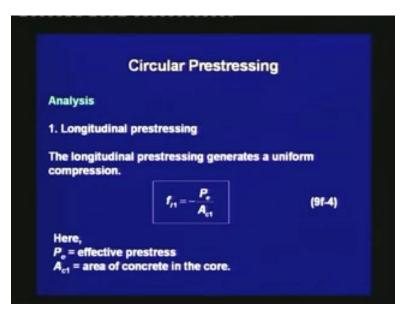
First is the longitudinal prestressing. The longitudinal prestressing generates a uniform compression which is given as  $f_{l1}$  is equal to minus  $P_e$  divided  $A_{c1}$ , where  $P_e$  is the effective prestress under service conditions and  $A_{c1}$  is the area of the concrete in the core.
