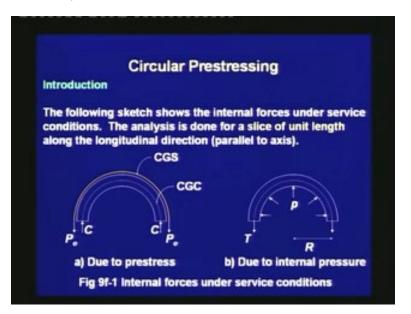
The following sketch shows the internal forces under service conditions. The analysis is done for a slice of unit length along the longitudinal direction, which is parallel to the axis of the member. In this sketch, the prestressing tendon is lying outside the shell and it is creating a hoop compression, where the compression is lying at the mid-plane of the shell, which is the CGC. Due to the internal pressure P, there is hoop tension which is also lying at the centre of the section.
