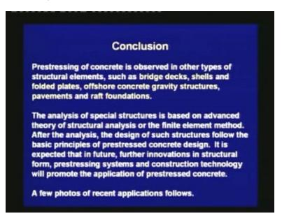
Finally, today we are concluding this prestressed concrete course. The prestressed concrete is observed in other types of structural elements, such as bridge decks, shells and folded plates, off shore concrete gravity structures and raft foundations.
