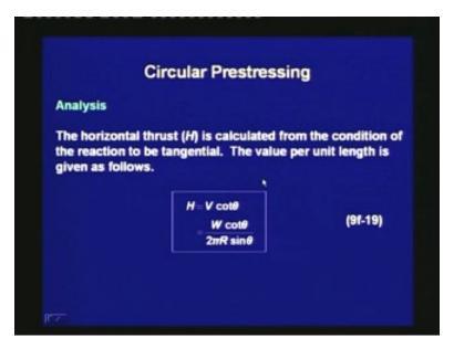
The horizontal thrust is calculated from the condition of the reaction to be tangential. The value per unit length is given as follows. H is equal to V cot theta is equal to W cot theta divided by 2 pi R sin theta.
