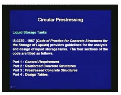
IS: 3370 – 1967; the title is Code of Practice for Concrete Structures for the Storage of Liquids, provide guidelines for the analysis and design of liquid storage tanks. The four section of the code are titled as follows: Part 1: General Requirement; Part 2: Reinforced
