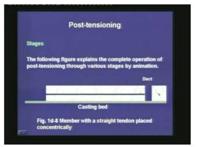
After the mould is placed, the concrete is cast with an annular space inside. This space is provided by placing a duct inside the concrete. After the casting of the concrete, when it has cured and hardened, a tendon is placed within the duct.
