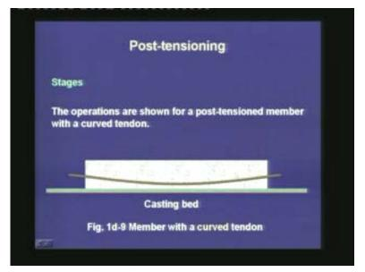
Once the concrete has cured and hardened, the tendon is passed through the duct, and the profile of the tendon becomes similar as the profile of the curved duct.
