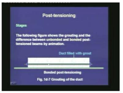
But if the annular space is filled up with grout then it is called a bonded post-tensioned beam.
