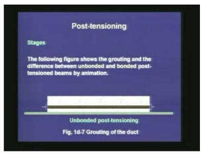
Let me show this once again. In this beam, the annular space between the tendon and the concrete is free of any grout and there is no direct stress transfer between the steel and the concrete along its length. The prestress is transferred only at the end anchorages.
