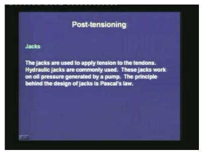
During the tensioning operation, the jacks are the most important equipment that we need. As I said, there can be several types of devices to apply the prestressing force. The most common is the hydraulic jacks which work on the principle of oil pressure. The design of these hydraulic jacks is based on Pascal's law.
