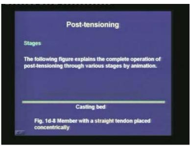
So, as I said in the post-tensioning, the casting bed need not be like a prestressing bed in the pre-tensioning system. The casting bed is just like any other ordinary casting yard.
