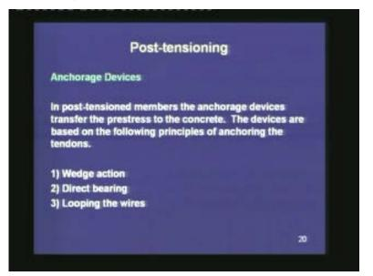
We shall move on to the anchorage devices for the post-tensioned beams. This is a very important device for the post-tensioning system because unless it is properly designed, it will not be able to transfer the prestress to the concrete. The anchorage devices are designed based on the following principles: the first is the wedge action, the second is the direct bearing against the concrete and the third is the looping of the wires.
