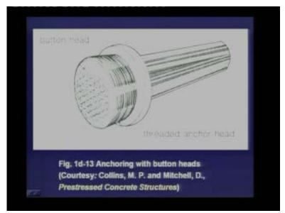
In this case, we can see that the individual wires have a button head, which is resting in the anchor head block. The anchor head is resting on the bearing plate, which rests against the concrete. This does not use the wedge action as shown before. Here, the button heads are just bearing against the anchor head, which is bearing against the plate, and which is further bearing against the concrete.
