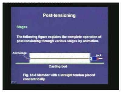
When the jack applies tension to the tendon, the concrete member undergoes elastic shortening. The tendon is subjected to the desired amount of tension, and then the jack can help the wedges to sit against the concrete member. Then the extra amount of the tendon is cut off from the two ends.
