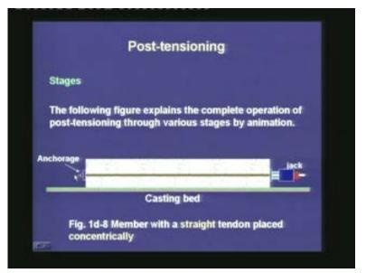
Then the end anchorage is placed at one end. On the other end, a jack is placed which gets reaction from the hardened concrete itself.
