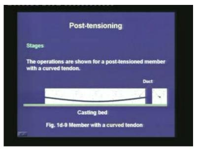
Now, in the casting bed after placing the mould, the concrete is cast with a curved duct inside it. Here, we can see that the profile of the duct is curved, which should be free of any obstacle.
