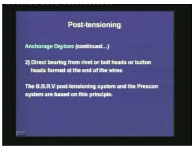
The second type of anchorage device is based on direct bearing from rivet or bolt holes or button heads formed at the end of the wires. Again, there are different types of patented system. The B.B.R.V post-tensioning system and the Prescon system are based on this principle of direct bearing of the button heads or the rivets against the concrete.
