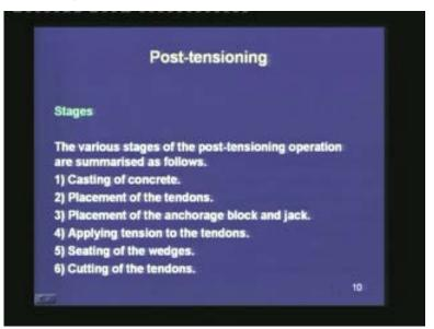
The various stages of the post-tensioning operation can be summarized as follows: first, the concrete is cast; it is allowed to cure and harden to achieve the desired strength before the tensioning operation is done. Next, the tendon is placed in the ducts which were
