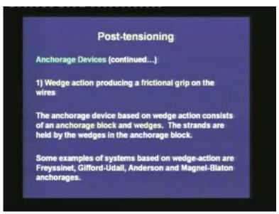
The anchorage device based on wedge action consists of an anchorage block, which is a substantially large block that can hold several wedges at a time. There are several individual wedges within the anchorage block. The strands are held by the wedges in the
