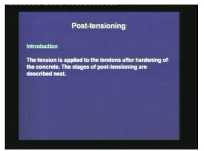
As we have mentioned earlier, prestressing can be broadly classified into two types: one is pre-tensioning and the other is post-tensioning. Post-tensioning is the one where the tension is applied to the tendons after hardening of the concrete. This is different from pre-tensioning. In pre-tensioning, the tension is applied first and then the concrete is cast. In our last lecture, we covered pre-tensioning in details. In this lecture, we shall cover post-tensioning and its devices.
