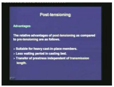
The post-tensioning operation has some advantages as compared to the pre-tensioning operation. First of all, the post-tensioning operation is suitable for heavy cast-in-place
