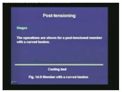
Next, we shall see the same operation for a post-tensioned beam, with a curved tendon. The curvature of a tendon is designed based on the bending moment the member will be subjected to in its service period. The curved profile is fixed by placing the duct appropriately with hangers within the reinforcement cage of the prestressing member.
