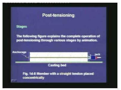
Once these are placed in position, the tension is applied by the jack and we can see as the jack applies tension, the concrete undergoes the elastic shortening. Before I go to the next one, let me show the previous animation once again.
