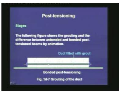
Next, if we fill the space with grout, after the grout hardens, then the steel and the concrete are bonded together, and then there can be stress transfer between the steel and
