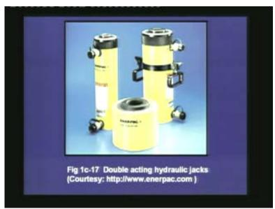
This photograph shows some double acting jacks. A double acting jack means that the piston can move in both the directions. There are two ports, an inlet and an outlet, for the oil. When oil enters through one port, the piston moves in one direction, and when the oil
