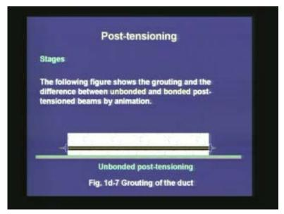
This figure will show the difference between a bonded tendon and unbonded tendon. In this sketch, you can see that the duct hole is free of any grout. We can see this black annular space which does not have any grout. If the beam is left just like this, then it is called an unbonded post-tensioned beam.
