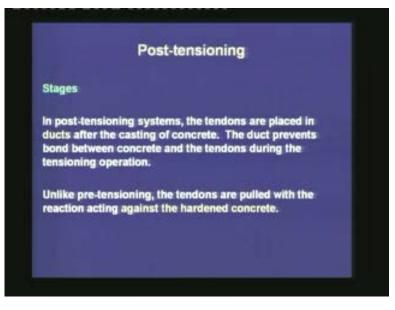
In post-tensioning systems, the tendons are placed in ducts after the casting of concrete. The duct prevents the bond between the concrete and the tendons during the tensioning operation. This is very essential because, when the tensioning operation is done if there is resistance, then the tension will not be applied properly. The duct ensures that there is no bond between the concrete and the steel during the tensioning process.
