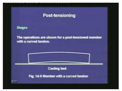
The jack gets the reaction from the hardened concrete. When it is applying the tension, since the tendon is curved, the member will have an upward displacement which is called cambering of a post-tensioned member. Due to the cambering, the member will hog up from the casting bed. Once the jacking operation is done, the extra amount of the tendons is cut off from the two ends.
