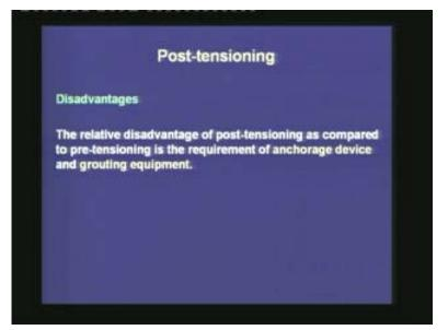
There are some disadvantages of post-tensioning as compared to pre-tensioning. The post-tensioning operation needs much more developed anchorage device as compared to pre-tensioning. In pre-tensioning, the anchorage devices are small. These are actually just some chuck assemblies for the individual strands; but in the post-tensioning operation, we shall see heavy-duty anchorage blocks for the transfer of prestress from the steel to the concrete.
