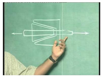
When the wedge is being pulled by the tendon, it gradually sits in this block and due to the friction action, the wedge is not able to move any further. Hence, the tension in the strands can be maintained by this wedge action, which acts on the principle of friction between these two blocks. Thus, the wedge action produces a frictional grip on the wires.
