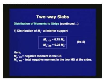
The first is that the distribution of  $M_u$  minus and interior support is as follows. For the column strip, it is 75% of  $M_u$  minus; for the middle strip on the two sides, total moment is 25% of the  $M_u$  minus. Remember that  $M_u$  minus MS is the total negative moment in the two middle strips in the 2 sides.
