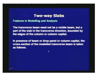
To account of this increased flexibility, as we move out from the column an equivalent column is defined in place of the actual column. The transverse beam need not be a visible beam, but a part of the slab in the transverse direction bounded by the edges of the column or column capital. In presence of beam or drop panel or column capital, the cross-section of the modelled transverse beam is taken as follows.
