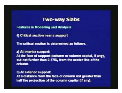
The fifth consideration is the defining the critical section near a support. The critical section is determined as follows. At an interior support, it is the face of support which is the column or column capital if any, but not further than  $0.175 l_1$  from the center line of the column. For an exterior support, it is at a distance from the face of column not greater than half the projection of the column capital, if any.
