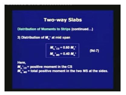
Third is a distribution of  $M_u$  plus at mid-span. The column strip gets 60% of the positive moment and the middle strip gets 40% of the positive moment. Again, note that for the middle strip, the  $M_u$  plus MS, represents the total positive moment in the two middle strip at the two sides.
