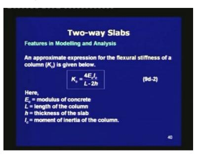
$K_c$  is equal to 4  $E_c$  times  $I_c$  divided by L minus 2 h. This is very close to the expression that we learnt from the slope deflection methods in basic structure analysis.  $E_c$  is the modulus of the concrete, L is the length of the column, h is the thickness of the slab and  $I_c$  is the moment of the inertia of the column. Thus, we have an expression of the flexural stiffness of a column which we can apply to the upper column and the lower column.
