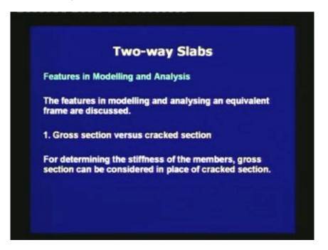
First is the gross section versus cracked section. The difficulty in analyzing a reinforced concrete structure is that the sections may become cracked if the load exceeds the service loads. The chances of cracking are reduced when the slabs are prestressed. The code allows us to use the gross cross-section instead of the cracked section which is difficult to find out. Thus for determining the stiffness of the members, gross section can be considered in place of cracked section.
