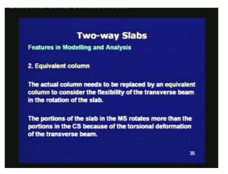
Second is the concept of equivalent column. The actual column needs to be replaced by an equivalent column to consider the flexibility of the transverse beam in the rotation of the slab. The portions of the slab in the middle strip rotate more than the portions in the column strip because of the torsional deformation of the transverse beam.
