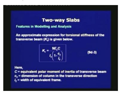
An approximate expression for the torsional stiffness of the transverse beam,  $K_t$  is given below.  $K_t$  is equal to 9 times  $E_c$  times C divided by  $I_2$  times, within bracket, 1 minus  $C_2$ divided by  $I_2$ . Here, C is the equivalent polar moment of inertia of transverse beam,  $C_2$  is the dimension of the column in the transverse direction,  $I_2$  is the width of the equivalent frame.
