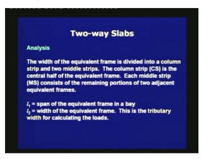
The width of the equivalent frame is divided into column strip and two middle strips. The column strip, which we denote as CS, is the central half of the equivalent frame. Each middle strip, which we shall denote as MS, consists of the remaining portions of two adjacent equivalent frames. In the following figure, we shall use  $l_1$  as a span of the equivalent frame in a bay;  $l_2$  as the width of the equivalent frame. This is the tributary width for calculating the loads.
