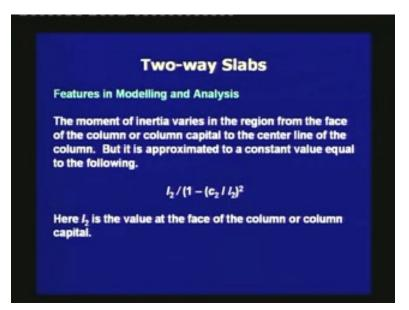
What values to be picked up is recommended by the code. Since the moment of inertia varies in the region from the face of the column or column capital to the center line of the column, it is approximated to a constant value equal to the following.  $I_2$  divided 1 minus  $C_2$ , divided by  $I_2$  the whole squared. Here,  $I_2$  is the value at the face of the column or column capital.
