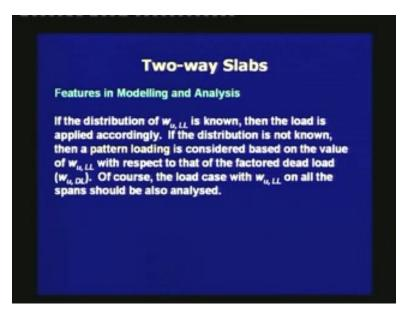
The coded recommendation is, if the distribution of  $W_{u,LL}$  is known, then the load is applied accordingly. If the distribution is not known, then a pattern loading is considered based on the value of  $W_{u,LL}$  with respect to that of the factored dead load  $W_{u,Dl}$ . The load case with  $W_{u,LL}$  on all the spans should be also analyzed.
