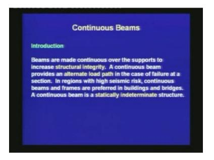
Beams are made continuous over the supports to increase structural integrity. A continuous beam provides an alternate load path in the case of failure at a section. In regions with high seismic risk, continuous beams and frames are preferred in buildings and bridges. A continuous beam is a statically indeterminate structure.
