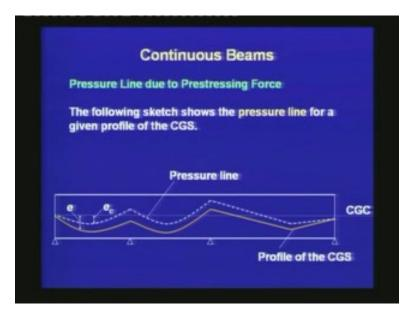
The orange line is the profile of the CGS and the dashed line is the pressure line. Observe that the pressure line has a similar variation as the profile of the CGS. Thus, due to the prestressing force the compression shifts up from the CGS to the pressure line. The important characteristics of the pressure line are as follows.
