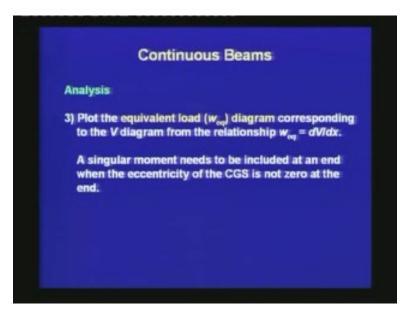
The third step is to plot the equivalent load or  $w_{eq}$  diagram, corresponding to the shear diagram from the relationship  $w_{eq}$  is equal to dV divided by dx. Thus, from the M<sub>1</sub> diagram we are calculating the shear force diagram; from the shear force diagram we are calculating the equivalent load diagram.
