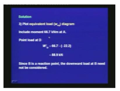
The point load at D is calculated from the change in the shear at the two ends and which gives a point load of 88.9 Kilonewtons. We are not considering an equivalent load at B, because B is a reaction point and the downward load at B need not be considered. The distributed load in the span BC is again calculated from the relationship,  $w_{eq}$  to dV divided by dx and from change in the shear diagram we are calculating  $w_{eq}$  is equal to 13.0 Kilonewtons per meter.
