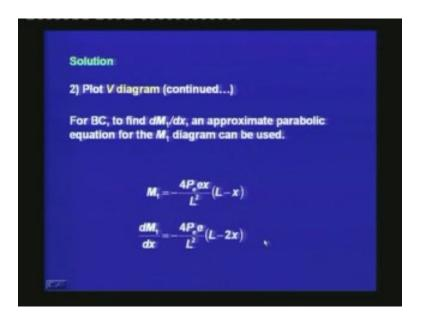
For BC, to find  $dM_1$  by dx, an approximate parabolic equation for the  $M_1$  diagram can be used.  $M_1$  can be expressed as a function of  $P_e$  and e as follows.  $M_1$  is equal to minus  $4P_e$  times e times x times within bracket L minus X divided by L square, from which we can find out an expression of  $dM_1$  by dx.
