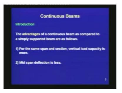
Next, the mid span deflection is less for continuous beam as compared to a simply supported beam. Since there is a strain at the two ends, the deflection at the middle is reduced in the continuous beam.
