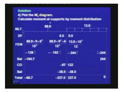
We are calculating the distribution factor, the fixed end moments for the given uniform load and then by the balance and carry over, we are calculating the total moments.
