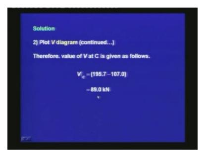
We are plotting the shear diagram and it is constant in AD, then DB, and it is linearly varying between B and C.
