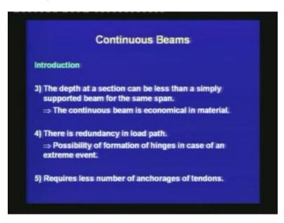
Third, the depth at a section can be less than a simply supported beam for the same span; that means, given the same span and same load, if we use a continuous beam it will have
