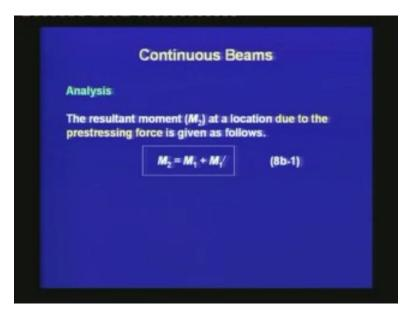
The resultant moment at a location due to the prestressing force is given as follows:  $M_2$  is equal to  $M_1$  plus  $M_1$  prime. In this equation,  $M_1$  is the moment due to prestressing force without the intermediate supports which is given as  $P_e$  times e.
