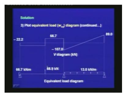
It has a point load, where the CGS has a short bend at D and it has a distributed load where the CGS has a parabolic variation in the span BC.
