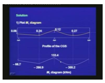
Thus, given the profile of the CGS, we are able to calculate the  $M_1$  diagram, which has
