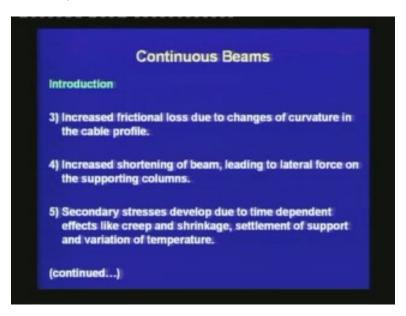
The third difficulty is increased frictional loss due to changes of curvature in the cable profile. If you have a cable running through the spans and the supports, there will be more changes in curvature and this will have increased frictional loss throughout the length of the beam. That is why at times the tendons are interrupted so as to reduce the frictional loss.
