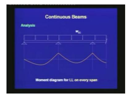
If the live load is uniform in all the spans, then the bending moment diagram is similar to that due to the dead load. It creates a positive moment in the end span, which is higher than the positive moment in the intermediate span and for the intermediate spans, the values of the negative moment is higher than that of the positive moment.
