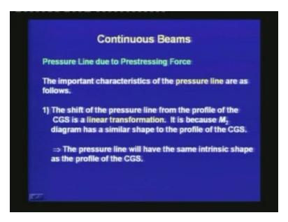
The shift of the pressure line from the profile of the CGS is a linear transformation. It is
