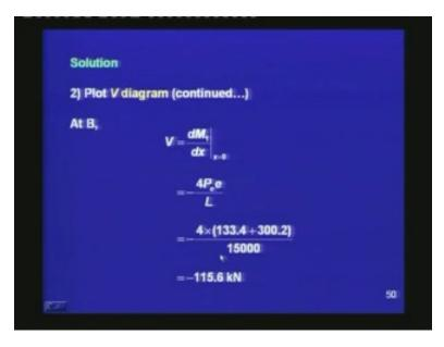
At B,  $dM_1$  by dx is calculated for x equal to 0, which is equal to  $4P_e$  times e divided by L
