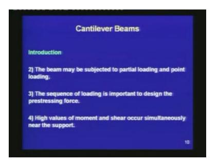
The second aspect is the beam may be subjected to partial loading and point loading. A cantilever beam, if it is subjected to a partial loading or a point loading, can generate a different type of moment condition as compared to when the load is distributed throughout. Hence, a partial loading or a point loading analysis becomes important for a cantilever.
