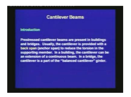
Prestressed cantilever beams are present in buildings and bridges. Usually, the cantilever is provided with a back span, which is also called anchor span, to reduce the torsion in the supporting member. In a building, the cantilever can be an extension of a continuous beam. In a bridge, the cantilever is a part of the balanced cantilever girder.
