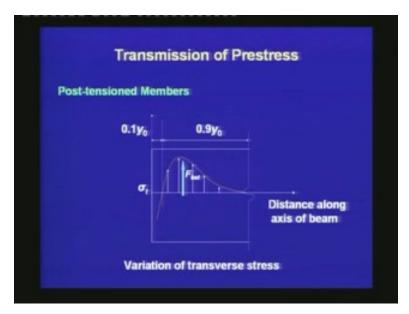
In our previous sketch, we have denoted the resultant of stresses by a force, which we denote as  $F_{bst}$  and this term is referred to bursting force. This force creates horizontal crack unless it is properly reinforced. This is called the splitting of the concrete. That means, splitting of the concrete refers to the horizontal crack that generates due to the stress concentration.
