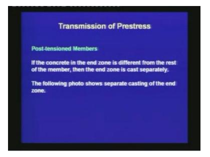
If the concrete in the end zone is different from the rest of the member, then the end zone is cast separately. The following photo shows separate casting of the end zone.
