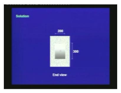
This is the design section for the bearing plate. The dimension of the bearing plate is 200 by 300 and it is placed concentrically with the end zone.
