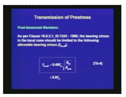
As per clause 18.6.2.1 of IS 1343-1980, the bearing stress in the local zone should be limited to the following allowable bearing stress, which is denoted as  $f_{br,allowable}$ . It is equal to 0.48  $f_{ci}$  times root over  $A_{br}$  divided by  $A_{punching}$ . The allowable bearing stress should be limited to 80% of  $f_{ci}$ .
