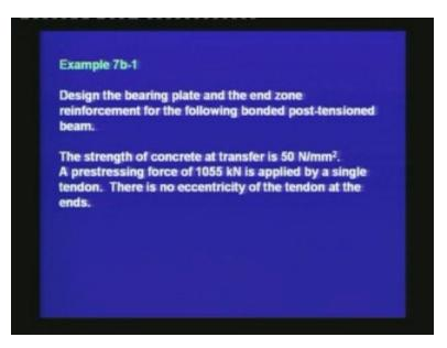
Let us now try to understand the design of the end zone reinforcement and the bearing plate by an example. Design the bearing plate and the end zone reinforcement for the following bonded post-tensioned beam. The strength of concrete at transfer is 50 Newton per millimeter square. A prestressing force of 1055 Kilonewtons is applied by a single tendon. There is no eccentricity of the tendon at the ends.
