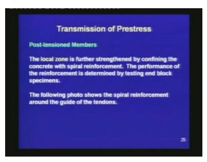
The local zone is further strengthened by confining the concrete with spiral reinforcement. Performance of the reinforcement is determined by testing end block specimens. The following photo shows the spiral reinforcement around the guide of the tendons.
