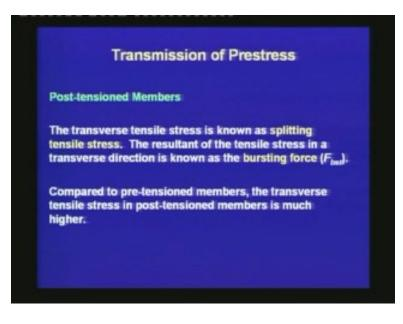
Compared to pre-tensioned members, the transverse tensile stress in post-tensioned members is much higher.
