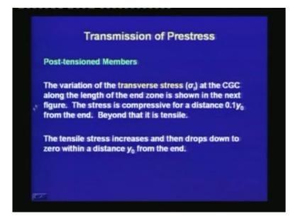
The variation of the transverse tensile stress sigma<sub>t</sub>, at the level of CGC along the length of the end zone is shown in the next figure. The stress is compressive for a distance  $0.1y_0$  from the end. Beyond that it is tensile. The tensile stress increases and then drops down to zero within a distance  $y_0$  from the end.
