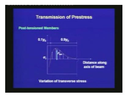
If you plot the variation of the transverse stresses at the level of CGC and along the axis of the beam, we observe that right behind the bearing plate, the transverse stresses are compressive. After a distance
