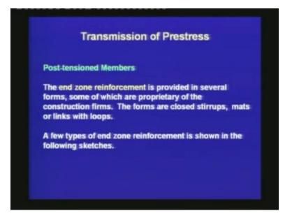
The end zone reinforcement is provided in several forms some of which are proprietary of the construction firms. The forms have closed stirrups, mats or links with loops. A few types of end zone reinforcement are shown in the following sketches.
