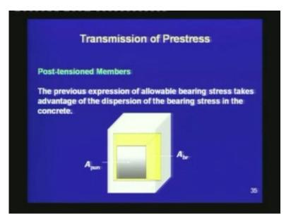
The previous expression of allowable bearing stress takes advantage of the dispersion of the bearing stress in the concrete.  $A_{punching}$  is the area where the bearing stress is applied and after that the bearing stress gets dispersed in the end zone to an area which can be placed within the end zone, this is geometrically similar to  $A_{punching}$ . Thus,  $A_{br}$  and  $A_{punching}$  are the two ends of a frustum which can be placed within the end zone.
