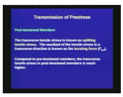
The transverse tensile stress is known as splitting tensile stress. The resultant of the tensile stress in a transverse direction is known as the bursting force.
