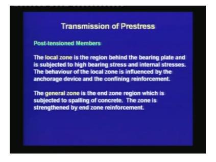
Thus, the local zone is the region behind the bearing plate and is subjected to high bearing stress and internal stresses. The behaviour of the local zone is influenced by the anchorage device and the confining reinforcement.
