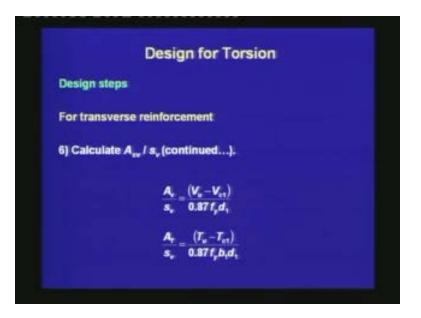
In the previous expression  $A_v/s_v$  is calculated from the shear to be carried by the steel which is  $(V_u - V_{c1})$ .  $A_T/s_v$  corresponds to the torsional shear that is to be carried by the steel which is  $(T_u - T_{c1})$ .
