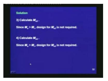
The third step is to calculate the next equivalent moment,  $M_{e2}$ . In this example,  $M_u$  is larger than  $M_t$  and hence design for  $M_{e2}$  is not required. The fourth step is to calculate  $M_{e3}$ . Here,  $M_u$  is larger than  $M_t$  and hence design for  $M_{e3}$  is not required.
