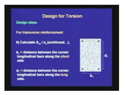
In the previous expression,  $b_1$  is the distance between the corner longitudinal bars along the short side, and  $d_1$  is the distance between the corner longitudinal bars along the long side. At the beginning, these values are not available exactly, but are estimated based on the cover requirement and estimated size of the transverse reinforcement.
