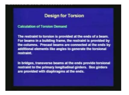
Next, we shall be discussing some general comments in the design for torsion. The restraint to torsion is provided at the ends of a beam. For beams in a building frame, the restraint is provided by the columns. Precast beams are connected at the ends by additional elements like angles to generate the torsional restraint.
