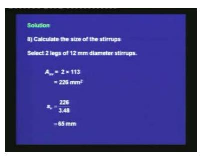
We are selecting the size as two legs of 12 mm diameter stirrups.  $A_{sv} = 2 \times 113 = 226$  mm<sup>2</sup>, from which we get  $s_v = 65$  mm.
