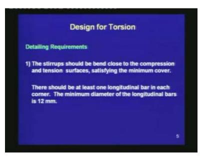
1) The stirrups should be bend close to the compression and tension surfaces, satisfying the minimum cover. There should be at least one longitudinal bar in
