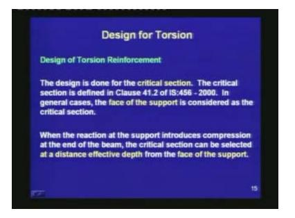
The design is done for the critical section. The critical section is defined in Clause 41.2 of IS: 456-2000. In general cases, the face of the support is considered as the critical section. When the reaction at the support introduces compression at the end of the beam, the critical section can be selected at a distance effective depth from the face of the support.
