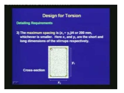
3) The maximum spacing of the stirrups is  $(x_1 + y_1)/4$  or 200 mm, whichever is smaller. Here,  $x_1$  and  $y_1$  are the short and long dimensions of the stirrups, respectively.
