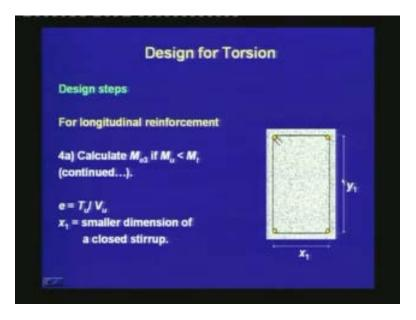
In the previous expression,  $e = T_u/V_u$ . Note that, this e is not the eccentricity of the prestressing steel. Here, e is the ratio of the ultimate torsional moment to the ultimate shear. For a closed stirrup, we are representing  $x_1$  as the smaller dimension and  $y_1$  as the larger dimension.
