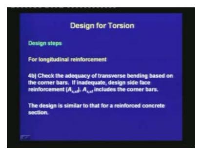
Once we have calculated  $M_{e3}$ , we need to check the adequacy of transverse bending based on the corner bars. If inadequate, design the side face reinforcement  $A_{s,sf}$ .  $A_{s,sf}$  includes the corner bars. The design is similar to that for a reinforced concrete section.
