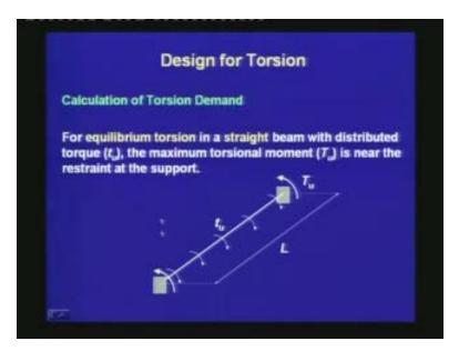
For equilibrium torsion in a straight beam with distributed torque  $t_u$ , the maximum torsional moment  $T_u$  is near the restraint at the support. This figure shows a beam, which is statically determinate and it is subjected to a distributed torque  $t_u$  per unit length. In this beam, the maximum torque comes at the two ends near the restraints at the supports and is denoted as  $T_u$ .
