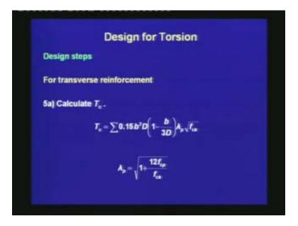
Next, we are moving on to the design of transverse reinforcement. The first step is to calculate the capacity of concrete to resist torsion.
