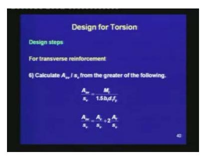
Now we are calculating the amount of transverse reinforcement from the greater of the two expressions of  $A_{sv}/s_v$ . The first expression is based on the skew bending theory, where  $M_t$  is the equivalent flexural moment.
