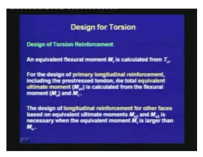
Next, an equivalent flexural moment  $M_t$  is calculated from  $T_u$ . For the design of primary longitudinal reinforcement, including the prestressed tendon, the total equivalent ultimate moment  $M_{e1}$  is calculated from the flexural moment  $M_u$  and  $M_t$ .
