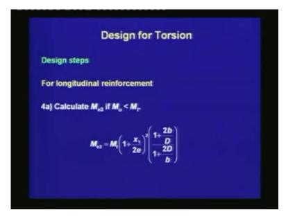
The fourth step is to calculate the third equivalent moment  $M_{e3}$  for transverse bending, if  $M_u$  is less than  $M_t$ . The expression of  $M_{e3}$  is given as follows.
