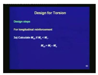
The third step is to calculate the other equivalent moment M<sub>e2</sub>, if M<sub>u</sub> is less that M<sub>t</sub>.
