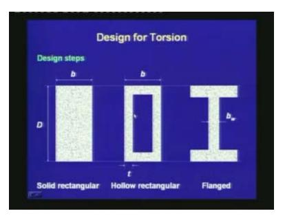
The geometric variables are defined for the different types of section as follows: b is the breadth which is the smaller dimension; D is the depth which is the longer dimension. For a hollow rectangular section, the thickness should be at least quarter of the breadth so that we have adequate shear flow zone. For a flanged section, the breadth of the web  $b_w$  substitutes b in the previous expression.
