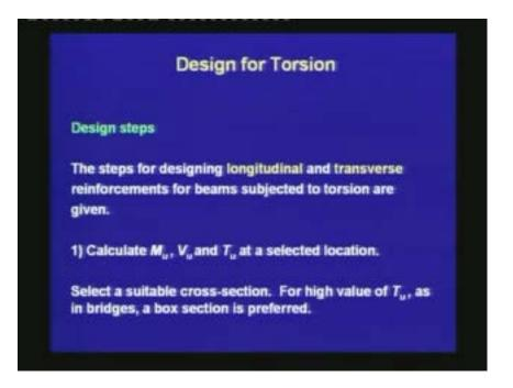
The steps for designing longitudinal and transverse reinforcement for beams subjected to torsion are given. First, calculate  $M_{u}$ ,  $V_{u}$  and  $T_{u}$  at a selected location. Select the suitable cross-section. For high value of  $T_{u}$ , as in bridges, a box section is preferred.
