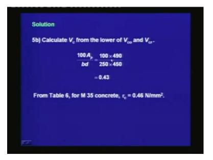
To calculate V<sub>c</sub>, we are first calculating the value of V<sub>cr</sub>. For that we need the amount of prestressing steel as a percentage.  $100A_p/bd = 100 \times 490/250 \times 450 = 0.43\%$  of prestressing steel. From Table 6, for M35 concrete,  $\tau_c = 0.46$  N/mm<sup>2</sup>.
