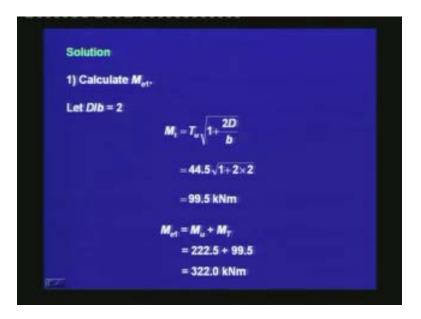
The first step is to calculate the equivalent moment  $M_{e1}$ . For the rectangular section, let the depth D divided by the breadth b is equal to 2; this gives an economical section. With this value of D/b we can calculate  $M_t$  from  $T_u$ .  $M_t = 99.5$  kNm. Thus,  $M_{e1} = M_u + M_t =$ 222.5 + 99.5 = 322 kNm.
