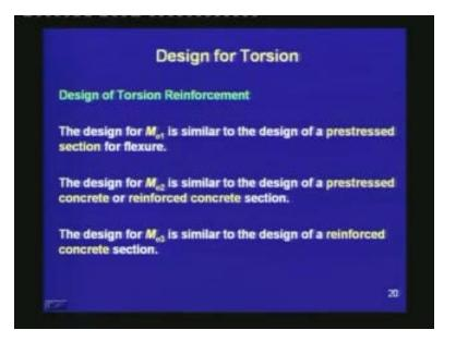
The design for  $M_{e1}$  is similar to the design of a prestressed section for flexure. Earlier in the chapter of design of members, we had studied in details, the design of members for flexure. In presence of torsion, once we calculate  $M_{e1}$  the design is exactly similar to what you have studied for flexure.
