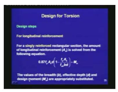
For a singly reinforced rectangular section, the amount of longitudinal reinforcement  $A_s$  is solved from the following equation.
