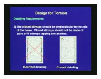
2) The closed stirrups should be perpendicular to the axis of the beam. Closed stirrups should not be made of pairs of U-stirrups lapping one another. As we had known earlier, for torsion we need close stirrups, to resist the circulatory shear.
