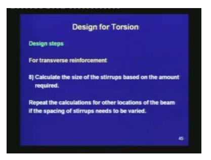
The eighth step is to calculate the size of the stirrups based on the amount required. Once we know  $s_v$ , we can calculate  $A_{sv}$  from the value of  $A_{sv}/s_v$ . From there, we calculate the size of the stirrups and the number of legs that will satisfy the value of  $A_{sv}$ .
