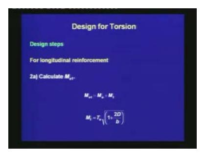
The next step is to calculate the equivalent moment  $M_{e1}$ .  $M_{e1}$  is equal to  $M_u + M_t$ , where  $M_t$  is calculated from the following expression.
