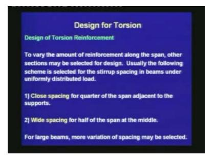
To vary the amount of reinforcement along the span, other sections may be selected for design. Usually, the following scheme is selected for the stirrup spacing in beams under uniformly distributed load: close spacing for quarter of the span adjacent to the supports; wide spacing for half of the span at the middle. For large beams, more variation of spacing may be selected.
