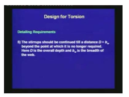
5) The stirrups should be continued till a distance  $D + b_w$  beyond the point at which it is no longer required. Here, D is the overall depth and  $b_w$  is the breadth of the web.
