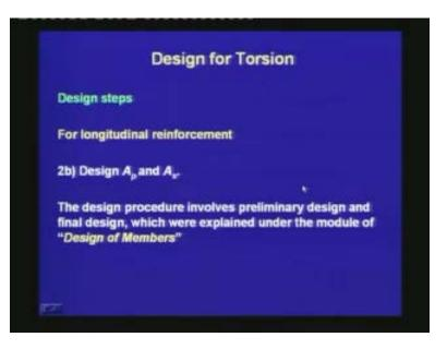
In the next step, we have to design  $A_p$  and  $A_s$ .  $A_p$  is the amount of prestressing steel and  $A_s$  is the amount of longitudinal steel. The design procedure involves preliminary design and final design, which were explained under the module of "Design of Members".
