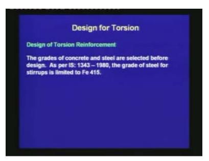
The grades of concrete and steel have to be selected before design. As per IS: 1343-1980, the grade of steel for stirrups is limited to Fe 415.
