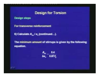
We have to satisfy the minimum amount of transverse reinforcement. The minimum amount of stirrups is given by the following equation.
