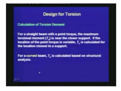
For a straight beam with a point torque, the maximum torsional moment  $T_u$  is near the closer support. If the location of the point torque is variable,  $T_u$  is calculated for the location closest to a support.
