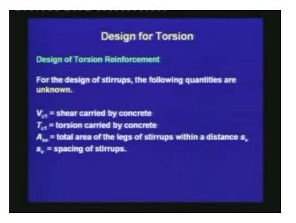
For the design of stirrups, the following quantities are unknown:  $V_{c1}$  is the shear carried by concrete;  $T_{c1}$  is the torsion carried by concrete;  $A_{sv}$  is the total area of the legs of stirrups within a distance  $s_v$ ; and  $s_v$  is the spacing of stirrups. Remember that  $T_{c1}$  and  $V_{c1}$ are the reduced values from the capacities of concrete under the individual actions.
