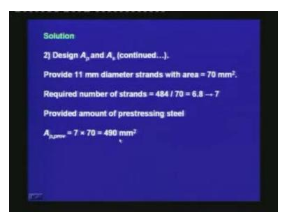
Provide 11 mm diameter strands with area 70 mm<sup>2</sup>. At this stage, we are selecting what type of strands we shall use for prestressing. The required number of strands is equal to  $484 \div 70 = 6.8$ , which is rounded off to 7. Provided amount of prestressing steel is  $A_{p,prov} = 7 \times 70 = 490 \text{ mm}^2$ . Thus, the amount of prestressing steel for the primary longitudinal reinforcement has been designed at the stage, and it is 7 of 11 mm diameter strands.
