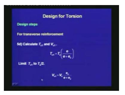
The parameters e and  $e_c$  are used in the interaction equation of the torsion and shear, from which we calculate the capacity of concrete to resist torsion and shear when both of them are acting together. In this step, we are calculating  $T_{c1}$  and  $V_{c1}$ .
