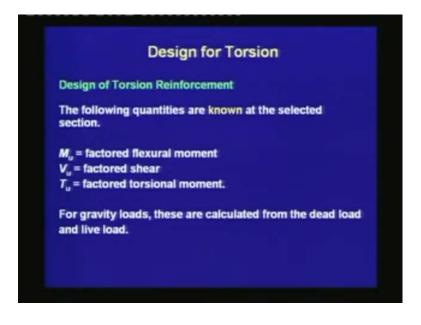
The following quantities are known at the selected section:  $M_u$  which is the factored flexural moment;  $V_u$  is the factored shear;  $T_u$  is the factored torsional moment. For gravity loads, these are calculated from the dead load and live load.
