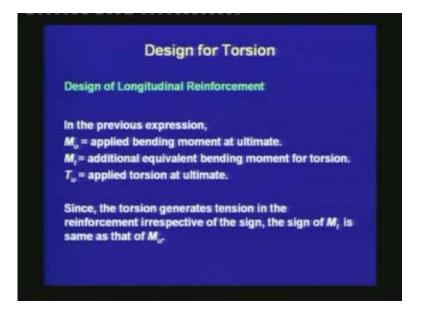
In this expression,  $M_u$  is the applied bending moment at ultimate;  $M_t$  is the additional equivalent bending moment for torsion;  $T_u$  is the applied torsion at ultimate. Since, the torsion generates tension in the reinforcement irrespective of the sign; the sign of  $M_t$  is same as that of  $M_u$ .
