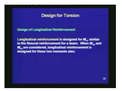
The longitudinal reinforcement is designed for  $M_{e1}$  similar to the flexural reinforcement for a beam. When  $M_{e2}$  and  $M_{e3}$  are considered, longitudinal reinforcement is designed for these two moments also.
