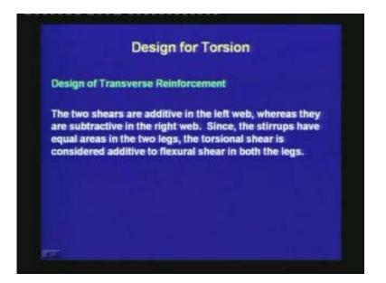
The two shears are additive in the left web whereas they are subtractive in the right web. Since, the stirrups have equal areas in the two legs, the torsional shear is considered additive to flexural shear in both the legs.
