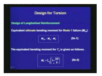
The equivalent ultimate bending moment for Mode 1 failure is denoted as  $M_{e1}$ .  $M_{e1} = M_u + M_t$ , where  $M_u$  is the ultimate flexural moment and  $M_t$  is the equivalent bending moment for the ultimate torsion.  $M_t = T_u \sqrt{(1 + (2D/b))}$ .
