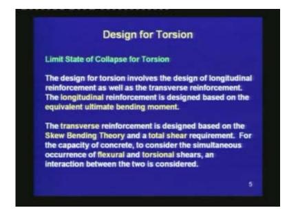
The design for torsion involves the design of longitudinal reinforcement as well as the transverse reinforcement. The resistance to torsion comes from a space truss action, where the concrete struts, the longitudinal steel and transverse reinforcement all take part in resisting the torsion. Hence, the design targets both the steel: longitudinal and transverse. For concrete, the design considers its capacity.
