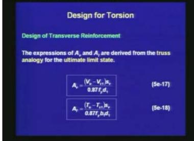
This expression is derived from the space truss analogy for torsion. Thus, once we know  $A_v$  and  $A_t$  we are combining them to get the value of  $A_{sv}$ , which is provided in the form of closed stirrups. Otherwise for a solid section, we can design for  $A_v$  and  $A_t$  separately.
