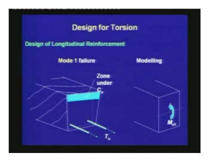
In the first mode of failure, there is an influence of the torsion on the bending. The plane of failure is skewed with the axis of the beam, but the zone of compression and the tension remain similar to conventional flexure. This is modeled by an equivalent moment which creates compression in the same face as that of the flexure, and it creates tension in the same phase as that of the flexure. (Refer Slide Time 08:34)
