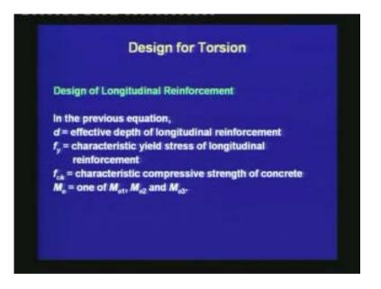
In this expression, d is the effective depth of longitudinal reinforcement,  $f_y$  is the characteristic yield stress of longitudinal reinforcement,  $f_{ck}$  is the characteristic compressive strength of concrete, and  $M_e$  is any of  $M_{e1}$ ,  $M_{e2}$  or  $M_{e3}$ .
