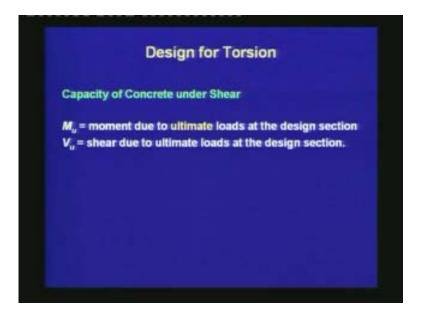
$M_u$  is the moment due to ultimate loads at the design section, and  $V_u$  is the shear due to ultimate loads at the design section.
