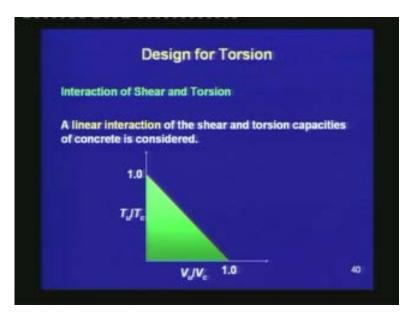
A linear interaction of the shear and torsion capacities of concrete is considered. In the graph, the ultimate shear  $V_u$  is normalized with the capacity of concrete to resist shear in the absence of torsion; this variable is in the x axis. In the y axis, the ultimate torsion  $T_u$  is normalized with respect to the capacity of concrete to resist torsion under pure torsion; this variable is plotted in the y axis.
