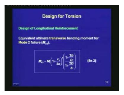
The equivalent ultimate transverse bending moment for Mode 2 failure is:
