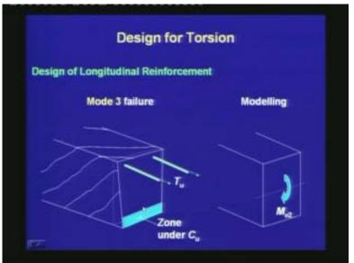
In this sketch, we can observe that the compression is occurring at the bottom and tension is at the top, which is in an opposite sense as that created by flexure. This is bending in an opposite sense to that of the flexural moment. This way, we check the requirement of the steel at the top.
