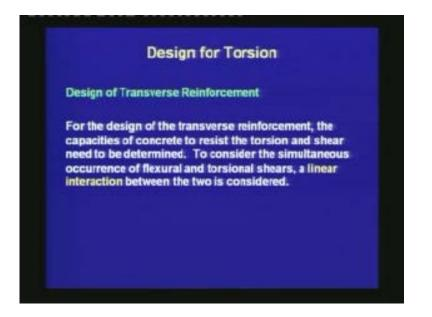
Next, is the design for transverse reinforcement. For the design of the transverse reinforcement, the capacities of concrete to resist the torsion and shear need to be determined. To consider the simultaneous occurrence of flexural and torsional shears, a linear interaction between the two is considered.
