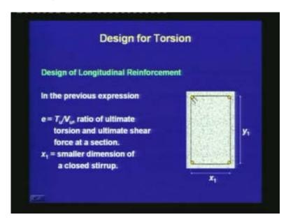
In this expression,  $e = T_u/V_u$ , ratio of ultimate torsion and ultimate shear force at a section,  $x_1$  is the smaller dimension of a closed stirrup. For a rectangular section, let  $x_1$  and  $y_1$  be the smaller and larger dimensions of the closed stirrup, respectively.
