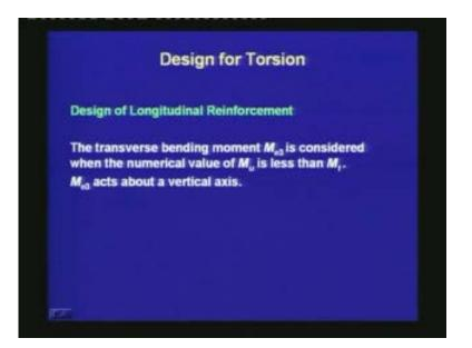
The transverse bending moment  $M_{e3}$  is considered when the numerical value of  $M_u$  is less than  $M_t$ .  $M_{e3}$  acts about a vertical axis.
