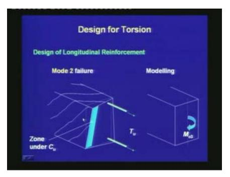
For the Mode 2 failure, the amount of torsion is significantly high and this type of failure is for beams with thin webs. Here, the compression of concrete is at one side face and the tension is in the other opposite side face. To model Mode 2 failure, the equivalent bending moment is considered to act about the vertical axis, which creates compression in one side face and tension in the other side face. For Mode 2 failure, the notation used in the codal expression is  $M_{e3}$ .
