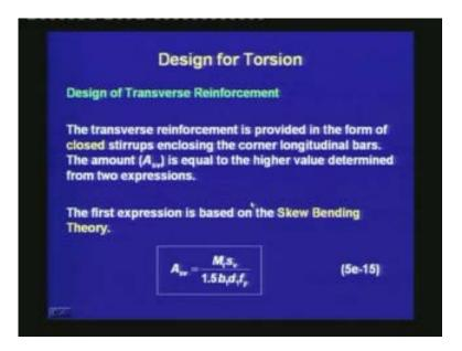
The transverse reinforcement is provided in the form of closed stirrups enclosing the corner longitudinal bars; this is the important requirement for the design for torsion. The torsion generates a circulatory shear, and hence the stirrups need to be closed. Open
