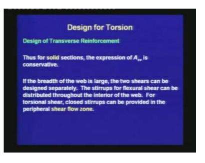
Thus for solid sections, the expression of  $A_{sv}$  is conservative. If the breadth of the web is large, the two shears can be designed separately. The stirrups for flexural shear can be distributed throughout the interior of the web. For torsional shear, closed stirrups can be provided in the peripheral shear flow zone. This is adopted to avoid clustering of the transverse reinforcement.
