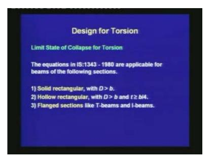
The equations in IS: 1343-1980 are applicable for beams of the following sections.
