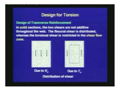
In solid sections, the two shears are not additive throughout the web. The flexural shear is distributed and acts downwards in the web, whereas the torsional shear is restricted in the peripheral shear flow zone; in one side it acts downwards, in the other side it acts upwards. In the central region, the shear is insignificant due to torsion. Thus, when shear and torsion act together they are not additive throughout the width of the web.
