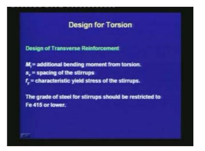
$M_t$  is the additional bending moment from torsion;  $s_v$  is the spacing of the stirrups;  $f_y$  is the characteristic yield stress of the stirrups. The grade of steel for stirrups should be restricted to Fe 415 or lower to have adequate ductility in the stirrups. Thus, we have found one expression of the transverse reinforcement, which is in terms of the equivalent moment due to torsion, and this is derived from the skew bending theory.
