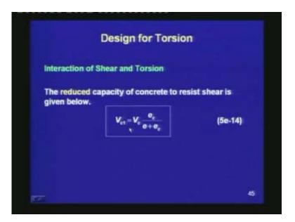
The reduced capacity of concrete to resist shear is given below.
