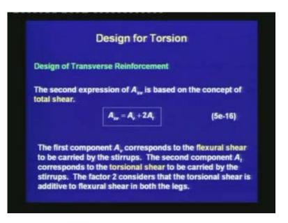
The second expression of A<sub>sv</sub> is based on a total shear requirement.
