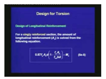
For a singly reinforced section, the amount of longitudinal reinforcement  $A_s$  is solved from the following equation.
