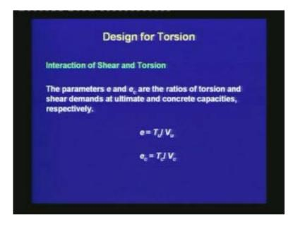
The parameters e and  $e_c$  are the ratios of torsion and shear demands at ultimate, and concrete capacities, respectively.
