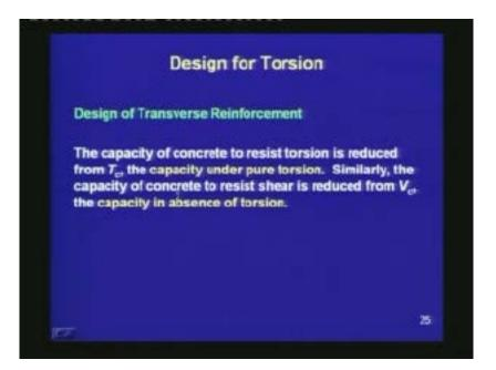
The capacity of concrete to resist torsion is reduced from  $T_c$ , the capacity under pure torsion. Similarly, the capacity of concrete to resist shear is reduced from  $V_c$ , which is the capacity in absence of torsion.
