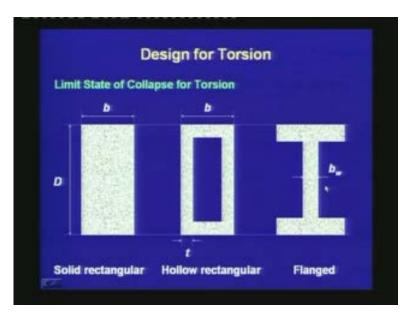
These are the three types of sections for which the equations are applicable. For a solid rectangular section D is larger than b. Similarly, for a hollow rectangular section, D is larger than b, and the thickness is greater than or equal to one quarter of b. For a flanged section, b has to be substituted by the breath of the web for most of the expressions.
