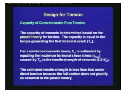
Next, we are developing the equation for the capacity of concrete under pure torsion, which will be represented as  $T_c$ . The capacity of concrete is determined based on the plastic theory for torsion. The capacity is equal to the torque generating the first torsional crack, which is represented as  $T_{cr}$ .
