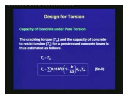
The cracking torque and the capacity of concrete to resist torsion, which is given as  $T_c$  for a prestressed concrete beam is thus estimated as follows:
