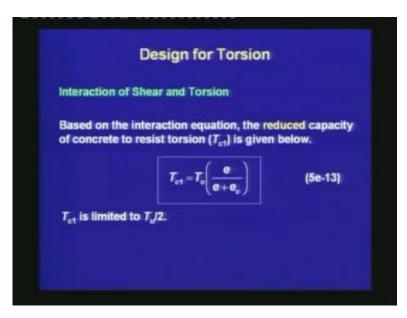
Based on the interaction equation, the reduced capacity of concrete to resist torsion, which is denoted as  $T_{c1}$ , is given below:
