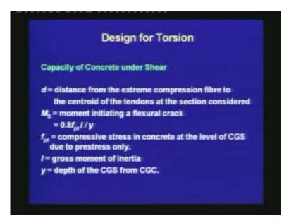
The other variables in the equation are: d is the distance from the extreme compression fibre to the centroid of the tendons at the section considered;  $M_0$  is the moment initiating a flexural crack which is estimated as  $0.8f_{pt}$  I/y;  $f_{pt}$  is the compressive stress in concrete at the level of CGS due to prestress only; I is the gross moment of inertia; y is the depth of the CGS from CGC.
