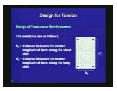
In this expression,  $b_1$  is the distance between the corner longitudinal bars along the short side;  $d_1$  is the distance between the corner longitudinal bars along the long side. Thus, for the rectangular section  $b_1$  is the shorter distance between the longitudinal bars and  $d_1$  is the larger distance between the longitudinal bars.
