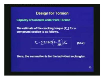
The estimate of the cracking torque T<sub>cr</sub> for a compound section is as follows.
