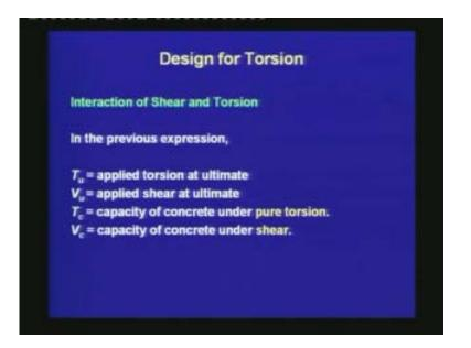
In this expression of the interaction equation:  $T_u$  is the applied torsion at ultimate;  $V_u$  is the applied shear at ultimate;  $T_c$  is the capacity of concrete under pure torsion;  $V_c$  is the capacity of concrete under shear.
