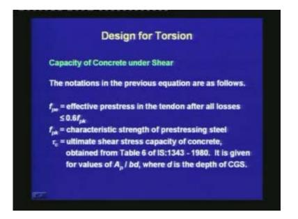
The notation in the previous equation are as follows:  $f_{pe}$  is an effective prestress in the tendon after all losses and it should be less than or equal to 0.6  $f_{pk}$ , where  $f_{pk}$  is the characteristic strength of prestressing steel;  $\tau_c$  is the ultimate shear stress capacity of concrete, obtained from Table 6 of IS: 1343 – 1980. It is given for values of  $A_p$ /bd, where d is the depth of CGS.
