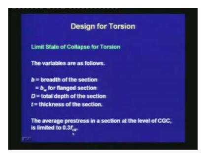
The variables are thus, b is the breath of the section which is equal to  $b_w$  for flanged section; D is the total depth of the section; t is the thickness of the section for a hollow section. The average prestress in a section at the level of CGC is limited to 0.3  $f_{ck}$ .
