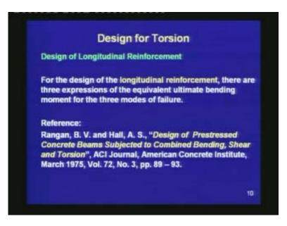
First, we are moving on to the design of longitudinal reinforcement. There are three expressions of the equivalent ultimate bending moment for the three modes of failure. We
