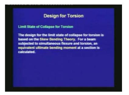
The design for the limit state of collapse for torsion is based on the skew bending theory. For a beam subjected to simultaneous flexure and torsion, an equivalent ultimate bending moment at a section is calculated.
