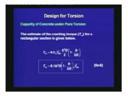
The estimate of the cracking torque  $T_{cr}$  for a rectangular section is given below.
