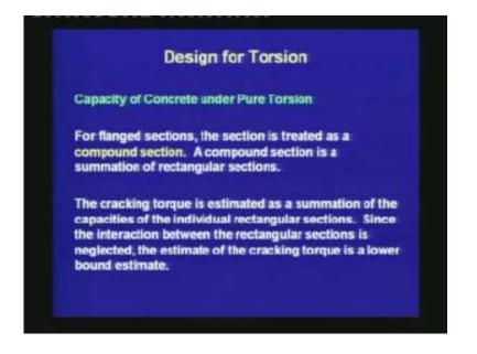
Now, the expression that we had seen was for a rectangular section. For a flanged section, the section is treated as a compound section. A compound section is a summation of rectangular sections.
