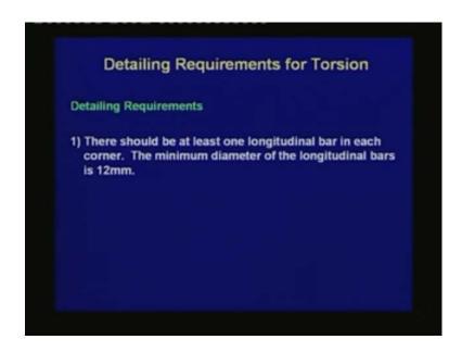
There should be at least one longitudinal bar in each corner. The minimum diameter of the longitudinal bars is 12 mm. Here, we see a requirement similar to the stirrups for shear that wherever we are bending the stirrups, we should provide a longitudinal bar that
