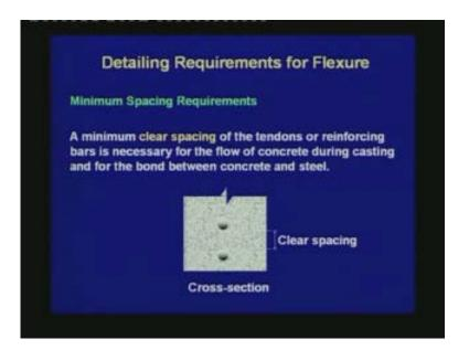
Next is the minimum spacing between the tendons. A minimum clear spacing of the tendons or reinforcing bars is necessary for the flow of concrete during casting and for the bond between concrete and steel. When we are talking of the clear spacing between the ducts, it is the spacing between the surfaces of the ducts.
