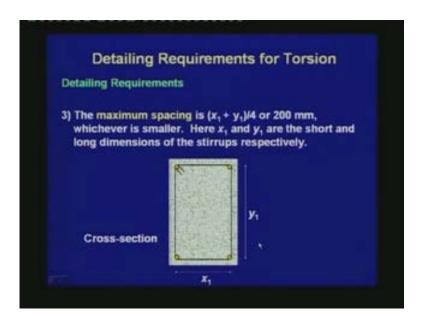
The maximum spacing of torsion reinforcement is  $(x_1 + y_1)/4$  or 200 mm, whichever is smaller. Here,  $x_1$  and  $y_1$  are the short and long dimensions of the stirrups, respectively. In this sketch,  $x_1$  is the horizontal dimension and  $y_1$  is the vertical dimension.
