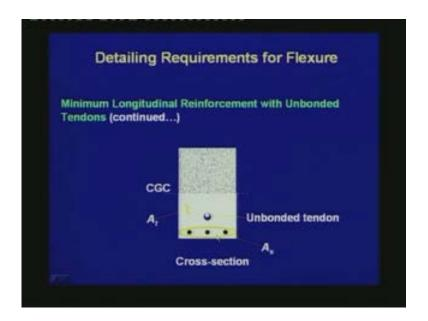
The way this reinforcement is calculated is that, we are considering the area which is under tension and that area is given by the part which is between the CGC and the extreme tension face. We are denoting that area by  $A_t$ . The minimum amount of non-prestressed reinforcement is equal to 0.4% of  $A_t$ .
