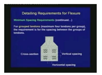
If we are grouping the tendons, then the requirement is for the spacing between the groups of tendons. The code allows having maximum 4 tendons in a group. In this sketch, we have shown 4 groups of tendons, where in each group there are 4 tendons. When we are referring to the spacing we are referring to the spacing between the groups. There is a requirement for a vertical spacing, and there is a requirement for a horizontal spacing.
