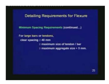
For large bars or tendons, the clear spacing should be greater than 40 mm. It should also be greater than the maximum size of tendon or bar, and it should also be greater than the maximum aggregate size + 5 mm.
