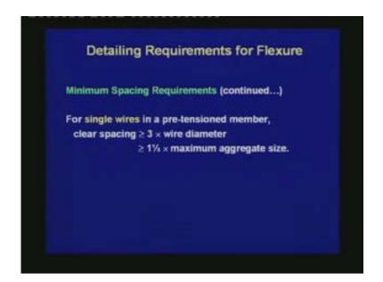
For single wires in a pre-tensioned member, the clear spacing should be greater than  $3 \times$  the wire diameter. It should also be greater than  $1\frac{1}{3} \times$  the maximum aggregate size.
