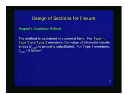
The method is explained in a general form. For Type 1, Type 2 and Type 3 members, the value of allowable tensile stress is properly substituted. For Type 1 member, the allowable tensile stress is 0. For Type 2 members, the allowable tensile stress is such that it is less than the cracking stress. For Type 3 members, the allowable tensile stress can be greater than the cracking stress, but the crack width should be limited, and hence there is an upper limit of the allowable tensile stress.
