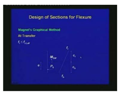
First, let us see the equations at transfer. The forces acting on the concrete section are the prestressing force  $P_0$  below the CGC, and the self-weight moment  $M_{sw}$ . The stress diagram across the depth of the section has a value of  $f_t$  at the top, which can be tensile and a value of  $f_b$  at the bottom, which is compressive. The distances of the top and the bottom from the CGC are denoted as  $c_t$  and  $c_b$ , respectively.
