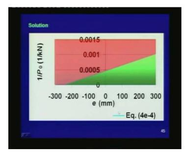
After plotting in the  $1/P_0$  versus e plane, the straight line passes through the point  $e = -k_t$ . Any point lying below this straight line is acceptable, and hence this region is shown as green; any point lying above the straight line is not acceptable, and that is shown in red.
