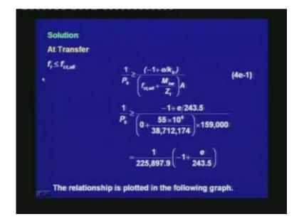
The first inequality relationship satisfies the condition that at transfer, the stress at the top should be less than the allowable tensile stress, which is  $f_{ct,all}$ . Since, it is a Type 1
