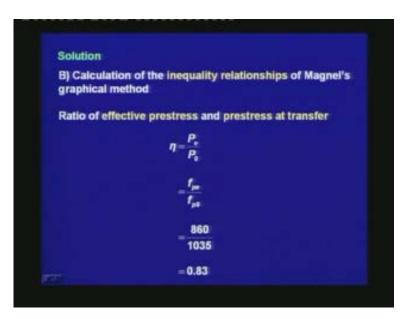
Next, we are calculating the inequality relationships from the stress conditions. The ratio of effective prestress and prestress at transfer  $\eta = P_e/P_0 = f_{pe}/f_{p0} = 860/1035 = 0.83$ . Thus, 83% of the prestress at transfer stays as the effective prestress.
