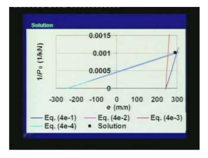
Once we plot all these four lines, we see that for this particular section, the allowable zone is a small strip on the right hand side; the solution is shown as a dark rectangle. Let us zoom into this small region which will show that the solution indeed lies in the acceptable zone.
