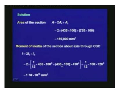
We are calculating the area of the section. Since,  $A_1$  is equal to  $A_3$ , the total area is given as  $2A_1 + A_2$ ;  $A_1$  is the flange width times the depth of the flange, which is  $435 \times 100$ ;  $A_2$ is equal to the remaining part of the depth of the web times the width of the web, which is  $720 \times 100$ . Once, we substitute the values the area is  $A = 159,000 \text{ mm}^2$ .
