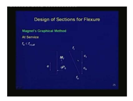
The fourth stress condition is that at service, the bottom stress  $f_b \le f_{ct,all}$ .
