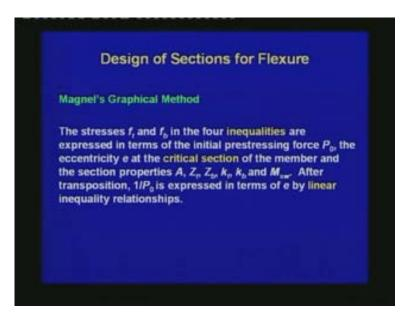
The stresses at the top and at the bottom in the four inequalities are expressed in terms of the initial prestressing force  $P_0$ , the eccentricity e at the critical section of the member and the section properties: area A, section moduli  $Z_t$ ,  $Z_b$ ; kern levels  $k_t$ ,  $k_b$ ; and self-weight moment  $M_{sw}$ . After transposition,  $1/P_0$  (the inverse of the prestressing force at transfer) is expressed in terms of the eccentricity e by linear inequality relationships.
