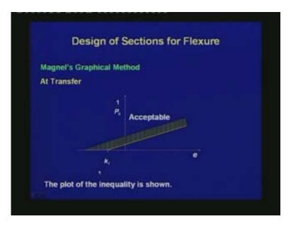
Hence, when we plot the corresponding straight line, it passes through the point  $e = -k_t$ . Since, in the equation  $1/P_0$  has to be greater than the value on the right hand side, any value above the straight line is acceptable.
