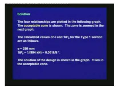
The four relationships are plotted in the following graph and the acceptable zone is shown. The zone is zoomed in the next graph. The calculated values of e and  $1/P_0$  for the Type 1 section, from the earlier design are as follows: e = 290 mm,  $P_0 = 994 \text{ kN}$ ,  $1/P_0 = 1/994 = 0.001 \text{ kN}^{-1}$ . The solution of the design is shown in the graph. It lies in the acceptable zone.
