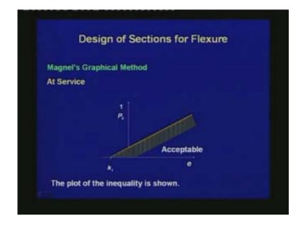
For this equation, we see that if  $e = -k_t$  then the numerator will be 0 and  $1/P_0 = 0$ . Hence, the straight line will pass through the point  $e = -k_t$ . The region below the straight line is
