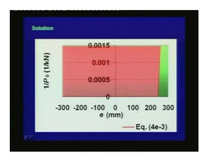
After plotting in the  $1/P_0$  versus e plane, the line passes through the point  $e = k_b$ . Any point which lies below the straight line is acceptable, here it is shown as green; and any point lying above the straight line is unacceptable, this is shown as red.
