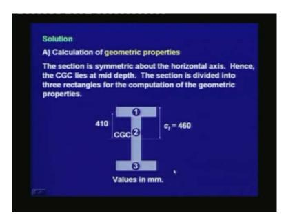
Here, we are checking the section based on the Magnel's method. First, we need to calculate the geometric properties of the section to plot the four lines in the  $1/P_0$  versus e plane.
