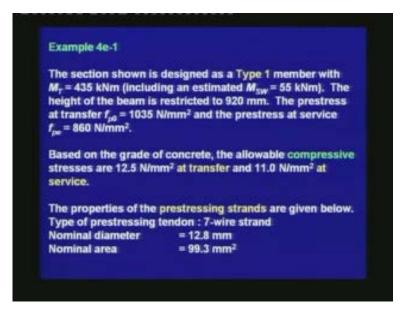
The section shown in the next slide, is designed as a Type 1 member with the total moment  $M_T = 435$  kNm, which includes an estimated self-weight of  $M_{sw} = 55$  kNm. The height of the beam is restricted to 920 mm. The prestress at transfer  $f_{p0} = 1035$  N/mm<sup>2</sup> and the prestress at service  $f_{pe} = 860$  N/mm<sup>2</sup>. Based on the grade of concrete, the allowable compressive stresses are 12.5 N/mm<sup>2</sup> at transfer and 11 N/mm<sup>2</sup> at service.
