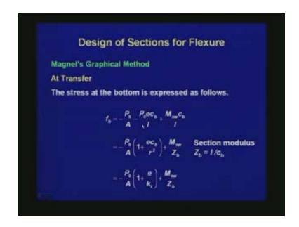
We are calculating the stress  $f_b$  just as before. It consists of the uniform component, which is  $-P_0/A$ . Then, it has the varying component  $(-P_0ec_b/I)$  which is due to the eccentricity of the prestressing force. Since the stress is compressive, we are placing a
