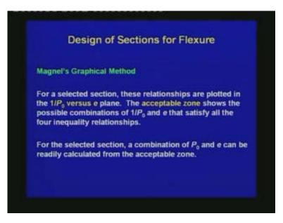
For a selected section, these relationships are plotted in the  $1/P_0$  versus e plane. The acceptable zone shows the possible combinations of  $1/P_0$  and e that satisfy all the four inequality relationships. For the selected section, a combination of  $P_0$  and e can be readily calculated from the acceptable zone.
