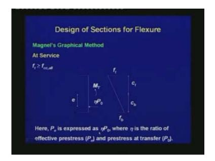
At service, we have to satisfy  $f_t \ge f_{cc,all}$ ; both these values are compressive and hence negative, and this equation is in an algebraic sense. At service, the prestressing force is denoted as  $\eta P_{0}$ , where  $\eta$  is a fraction of the initial prestressing force. The prestressing force has reduced due to the long-term losses.  $M_T$  is the total moment due to the dead load and live load.
