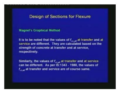
It is to be noted that the values of  $f_{cc,all}$  at transfer and at service are different. They are calculated based on the strength of concrete at transfer and at service, respectively. Similarly, the values of  $f_{ct,all}$  at transfer and at service can be different. As per IS:1343 – 1980, the values of  $f_{ct,all}$  at transfer and at service have been made same based on the reason that the values are small.
