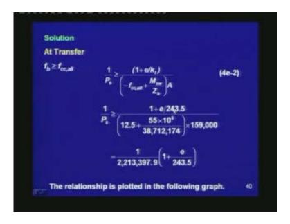
The second condition is at transfer, the stress at the bottom should be greater than the compressive stress at transfer. After substituting the values of  $k_t$ ,  $M_{sw}$ ,  $Z_b$  and A, the corresponding relationship is  $1/P_0 \ge 1/2,213,397.9 \times (1 + e/243.5)$ .
