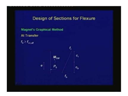
The second stress condition at transfer is that  $f_b \ge f_{cc,all}$  in an algebraic sense, because both these values are negative.
