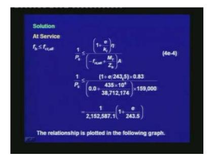
Next, we are moving on to the fourth condition which states that the stress at the bottom should be less than the allowable tensile stress at service. In the corresponding equation,
