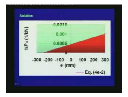
When we plot this relationship, the line passes through the point  $e = -k_t = -243.5$  mm. As before, the straight line demarcates the  $1/P_0$  versus e plane into two regions. Any combination which lies above the straight line is acceptable, and that is shown as green; any combination lying below the straight line is not acceptable, which is shown as red.
