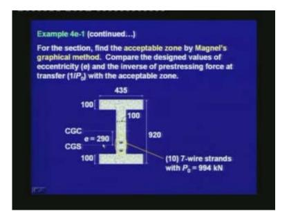
For the section, find the acceptable zone by Magnel's graphical method. Compare the designed values of the eccentricity e and the inverse of prestressing force at transfer (which is  $1/P_0$ ) with the acceptable zone.
