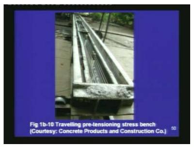
This is a travelling pre-tensioning stress bench. It is called a stress bench because the tendons are anchored to this unit, and this unit can move from one place to another on the rollers which are placed in rails. Hence, this is called a travelling pre-tensioning stress bench.
