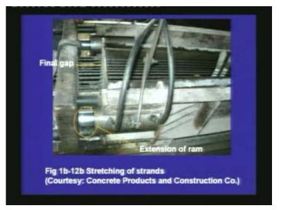
This is the situation after the tendons have been stretched. Note that the piston of the jack has come out. It has pushed the end plate to extend the tendons. The gap between the end plate and the end of the stress bench has increased.
