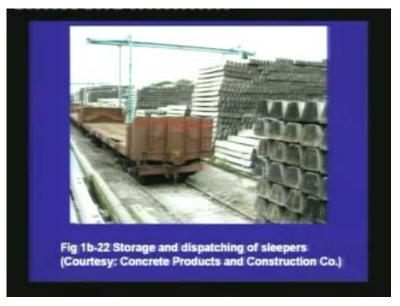
In the above photograph, we can see that from the stacking yard, the sleepers are being loaded onto wagons. These will be transported to the site where they will be placed beneath the rails. Thus, the pre-tensioning operation is a very fast track construction, and it is suitable for mass production of prestressed elements like railway sleepers, poles and other smaller units. This is done in a controlled environment with proper quality control and precise tensioning of the tendons.
