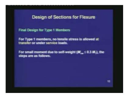
To recollect, for Type 1 members no tensile stress is allowed at transfer or under service loads. For small moment due to self-weight, say  $M_{sw}$  less than 30% of the total moment, the steps are as follows.
