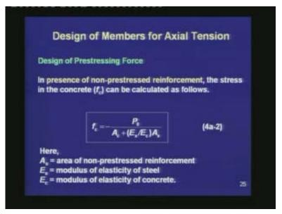
If we have non-prestressed reinforcement in addition to prestressing tendon, the stress in the concrete can be calculated as follows:  $f_c = -P_0 / (A_c + (E_s/E_c)A_s)$ .  $A_s$  is the area of non-prestressed reinforcement,  $E_s$  is the modulus of elasticity of steel, and  $E_c$  is the modulus of elasticity of concrete.
