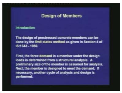
First, we shall study the design of members in general. For design of prestressed concrete members, we follow the limit states method as given in Section 4 of IS: 1343-1980. First, the force demand in a member under the design loads is determined from a structural analysis. A preliminary size of the member is assumed for analysis. Next, the member is designed to meet the demand. If necessary, another cycle of analysis and design is performed.
