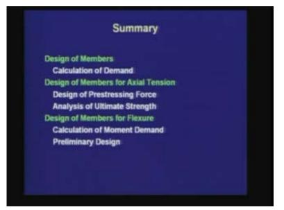
In this lecture, we started to learn about the design of members. First, we studied how to calculate the demand in the member. We need to have the characteristic values of the loads to start with. The characteristic values for dead load, live load, wind load and snow load are available from IS: 875. The earthquake load is available from IS: 1893 Part 1.
