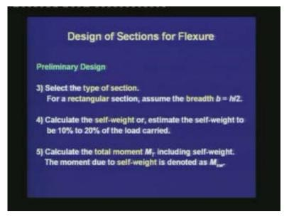
The third step in the preliminary design is to select the type of section. There can be several types of sections depending on the applications. We shall learn more about them in our subsequent lecture. For a rectangular section, which is the simplest type of section, we can assume the breadth b is equal to half of the total depth.
