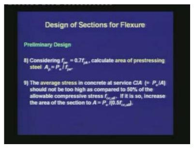
The eighth step is, considering the effective prestress  $(f_{pe})$  is equal to 70% of the characteristic tensile strength of the prestressing steel, calculate area of prestressing steel  $A_p = P_e/f_{pe}$ . At this stage, we are estimating the area of the prestressing steel based on the estimate of the prestressing force and the effective prestress.
