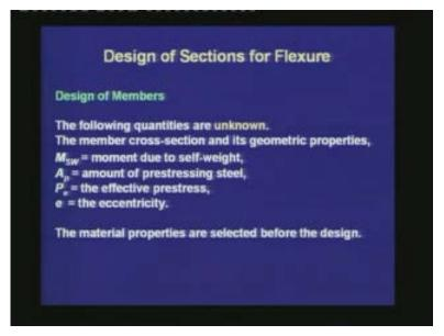
The following quantities are unknown: the member cross-section and its geometric properties. We do not know  $M_{SW}$ , the moment due to self-weight of the member. The other unknown quantities are:  $A_p$  the amount of prestressing steel,  $P_e$  the effective prestress, and e the eccentricity of the CGS at the critical section. Thus, the unknown quantities are in fact, more than the available set of equations.
