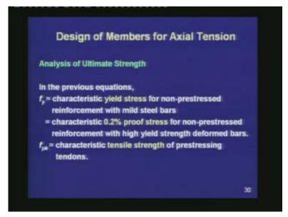
Here,  $f_y$  is the characteristic yield stress for non-prestressed reinforcement with mild steel bars, or it is the characteristic 0.2% proof stress for non-prestressed reinforcement with high yield strength deformed bars;  $f_{pk}$  is the characteristic tensile strength of prestressing tendons.
