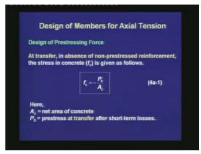
At transfer, in the absence of non-prestressed reinforcement, the stress in concrete, which is denoted as  $f_c$  is given as follows:  $f_c = -P_0 / A_c$ . Here,  $A_c$  is the net area of the concrete that we have studied earlier, and  $P_0$  is the prestress at transfer after short-term losses. We are denoting the negative stress for compression.
