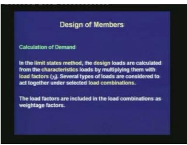
In the limit states method, the design loads are calculated from the characteristic loads by multiplying them with load factors, which are represented as  $\gamma_f$ . Several types of loads are considered to act together under selected load combinations. The load factors are included in the load combinations as weightage factors.
