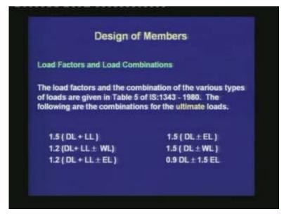
Next, the load factors and the combination of the various types of loads are given in Table 5 of IS: 1343-1980. The following are the load combinations for the ultimate loads:
