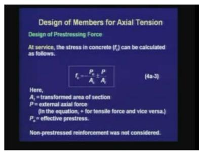
Next, we are moving on to the analysis of stresses for service loads. At service, the stress in concrete can be calculated as follows:  $f_c = -P_e/A_c \pm P/A_t$ . Here,  $A_t$  is the transformed area of the section, P is the external axial force (in the equation, + is used for tensile force
