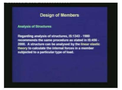
Regarding analysis of structures, IS: 1343-1980 recommends the same procedure as stated in IS: 456-2000. A structure can be analyzed by the linear elastic theory to calculate the internal forces in a member subjected to a particular type of load. Thus, the code allows us to use the linear elastic theory for the analysis, even if we do the design based on the limit states method.
