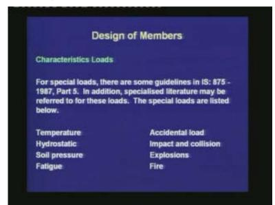
For special loads, there are some guidelines in IS: 875-1987 Part 5. In addition, specialized literature may be referred to for these loads. The special loads are listed below: Temperature, hydrostatic, soil pressure, fatigue, accidental load, impact and collision, explosions and fire. Thus, we see that for the special loads, IS: 875 Part 5 gives us some basic guidelines, but we may need specialized literature or international codes to get more detailed values for these special loads.
