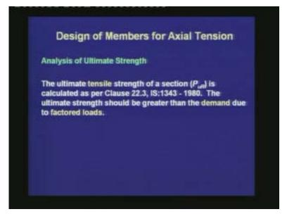
The ultimate tensile strength of a section, which is represented as  $P_{uR}$ , is calculated as per Clause 22.3 of IS: 1343-1980. The ultimate strength should be greater than the demand due to factored loads.
