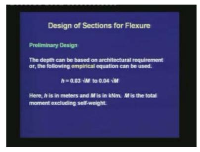
The selection of the depth of a beam usually is governed by the architectural requirement, depending on the required clearance beneath the beam. If the architectural requirement is not given, then a preliminary estimate of the depth can be based on the following empirical equation.  $h = 0.03 \sqrt{M}$  to  $0.04 \sqrt{M}$ . Here, h is in meters and M is in kNm. M is the total moment excluding self-weight.
