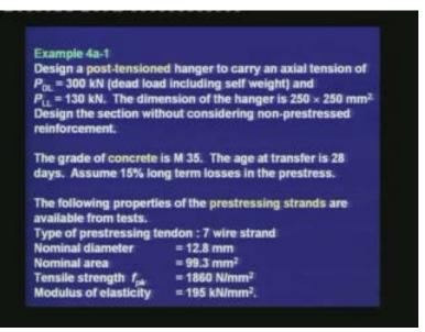
Design a post-tensioned hanger to carry an axial tension of  $P_{DL} = 300$  kN (the dead load includes the self-weight) and  $P_{LL} = 130$  kN. The dimension of the hanger is  $250 \times 250$  mm<sup>2</sup>. Design the section without considering non-prestressed reinforcement. The grade of concrete is M35, and the age at transfer is 28 days. Assume 15% long-term losses in the prestress.
