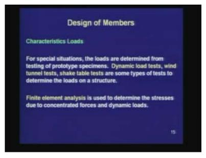
For special situations, the loads are determined from testing of prototype specimens like dynamic load tests, wind tunnel tests, shake table tests or some type of tests to determine the loads on a structure. Finite element analysis is used to determine the stresses due to concentrated forces and dynamic loads.
