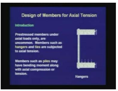
Next, we move on to design of members for axial tension. Prestressed members under axial tension only, are uncommon. Members such as hangers and ties are subjected to axial tension. Members such as piles may have bending moment along with axial compression or tension. In this figure, we see a hanger, where only the forces in the vertical direction have been shown. This hanger can be prestressed to have no tension in the concrete under the service loads.
