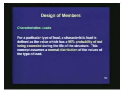
Next, let us study that for a particular type of load, a characteristic load is defined as a value which has 95% probability of not being exceeded during the life of the structure. This concept assumes a normal distribution of the values of the type of load.
