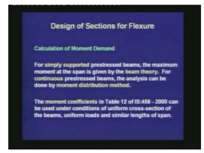
For flexure, how do we calculate the moment demand? For simply supported prestressed beams, the maximum moment at the span is given by the beam theory. For continuous prestressed beams, the analysis can be done by the moment distribution method. The moment coefficients in Table 12 of IS: 456-2000 can be used under conditions of uniform cross-section of the beams, uniform loads and similar lengths of span.
