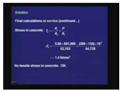
The stress in concrete due to service loads is given as  $f_c = -P_e/A_c + P/A_t$ . The value of  $P_e$  is equal to 85% of the prestress at transfer. The external force is 300 (the dead load)
