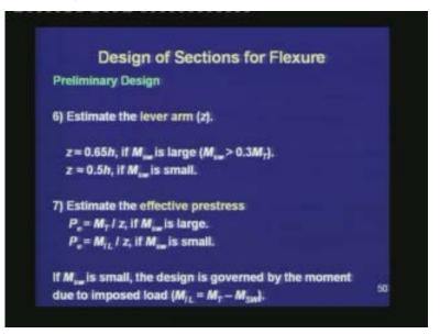
We are estimating the lever arm for the preliminary design. The lever arm z is roughly equal to 0.65 times h, if  $M_{sw}$  is large ( $M_{sw}$  greater than 30% of the total moment). If  $M_{sw}$  is small, then the lever arm can be taken as half of the total depth.
