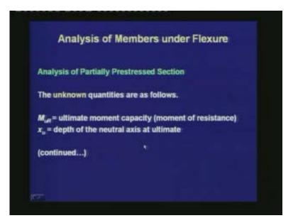
What are the unknown quantities? The first unknown quantity is  $M_{uR}$  which is the ultimate moment capacity. The second unknown quantity is  $x_u$ , the depth of the neutral axis at ultimate.
