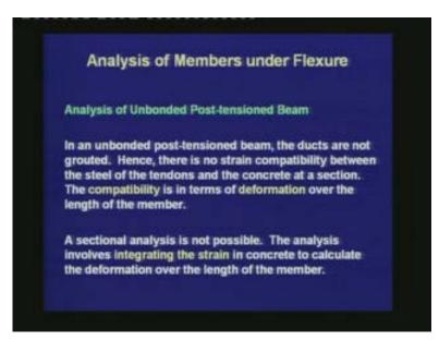
In an unbonded post-tensioned beam, the ducts are not grouted. Hence, there is no strain compatibility between the steel of the tendons and the concrete at a section. The compatibility is in terms of deformation over the length of the member. A sectional analysis is not possible. The analysis involves integrating the strain in concrete to calculate the deformation over the length of the member.
