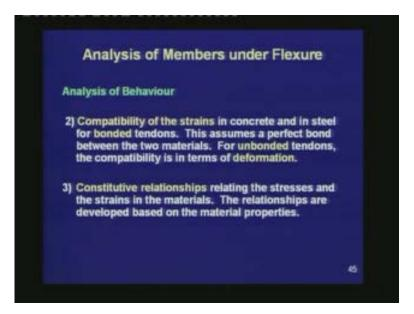
The second principle that we use is the compatibility of the strains in concrete and in steel for bonded tendons. This assumes a perfect bond between the two materials. Thus, to relate the strains in the several layers of steel with the strain in the concrete, we use the strain compatibility equations. If we have unbonded tendon, then the strain compatibility equation cannot be used. For an unbonded tendon, we use the compatibility in terms of deformation.
