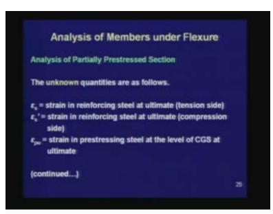
We do not know the strains in the steel at ultimate:  $\varepsilon_s = \text{strain}$  in reinforcing steel for the tension side,  $\varepsilon_s' = \text{strain}$  in the reinforcing steel for the compression side,  $\varepsilon_{pu} = \text{strain}$  in the prestressing steel at the level of CGS.
