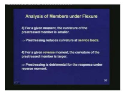
The third observation is for a given moment, the curvature of the prestressed member is smaller.
