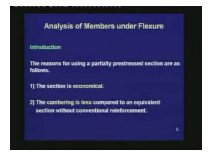
What are the reasons for using a partially prestressed section? The reasons are as follows. First, a partially prestressed section is economical compared to a fully prestressed section. We do not need as much amount of prestressing steel and anchorage units as compared to a fully prestressed section.
