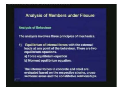
The analysis involves three principles of mechanics: first, the equilibrium of internal forces with the external loads at any point of the behavior. There are two equilibrium equations: a) force equilibrium equation, b) moment equilibrium equation.
