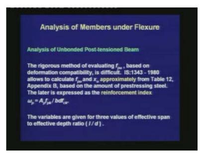
The rigorous method of evaluating  $f_{pu}$ , based on deformation compatibility is difficult. IS: 1343-1980 allows the calculation of  $f_{pu}$  and  $x_u$  approximately from Table 12 Appendix B, based on the amount of prestressing steel. The later is expressed as the reinforcement index  $\omega_p = A_p f_{pk}/bdf_{ck}$ . The variables are given for three values of effective span to effective depth ratio, which is denoted as l/d.
