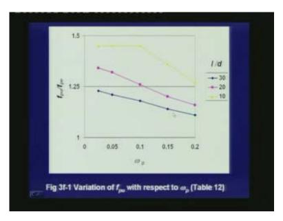
As we had seen for bonded tendons, the code allows us to use some approximate values for  $x_u$  and  $f_{pu}$ , based on the reinforcement index. In the tables for a bonded tendon,  $f_{pu}$  is normalized with respect to  $0.87f_{pk}$ , the maximum allowed stress in the tendon. In the tables for an unbonded tendon,  $f_{pu}$  is normalized with respect to  $f_{pe}$ , the effective prestress.
