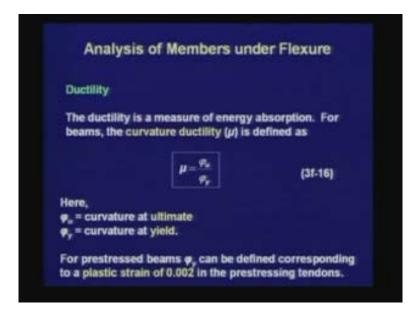
For beams, we define the ductility in terms of curvature and we are denoting it as  $\mu$ . The curvature ductility is the ratio of the curvature at ultimate which is denoted as  $\phi_u$ , divided by the curvature at yield which is denoted as  $\phi_y$ . When we are designing for seismic forces, the ductility becomes an important consideration.
