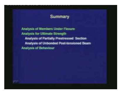
Today we studied the analysis for ultimate strength of a partially prestressed section. A beam may not be fully prestressed. There can be conventional reinforcement along with the prestressing tendon. There are some advantages of partially prestressed sections. First of all, the sections are economical. Next, the sections have more ductility. It is better for reversal of moments. In a beam with unbonded tendons, in presence of bonded reinforcement, the cracks are more distributed.
