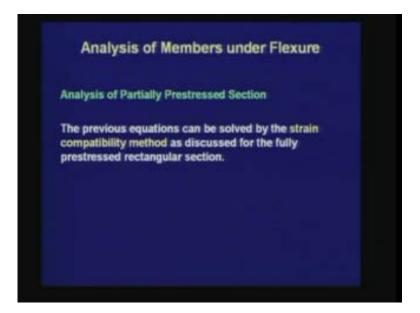
The set of equations can be solved iteratively by the method of strain compatibility, as we have learnt for a fully prestressed section.
