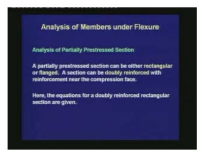
A partial prestressed section can be analyzed either as a rectangular or a flanged section. In our previous lectures, we have studied the analysis of fully prestressed sections for rectangular and flanged sections. We analyze a section as a flanged section, when the flanges are in compression and the depth of neutral axis is larger than the depth of the flange. In a partially prestressed section also, we can have either a rectangular section or a flanged section.
