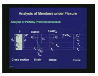
In the analysis for ultimate state, first we start with the strain diagram. The failure is defined as when the strain in the extreme compression fibre is equal to 0.0035. A linear strain diagram is drawn based on the principle, plane sections remain plane till ultimate.
