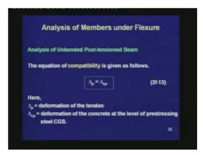
$\Delta_p = \Delta_{cp}$ , where  $\Delta_p$  is the deformation of the tendon and  $\Delta_{cp}$  is the deformation of the concrete at the level of prestressing steel, which is the CGS.
