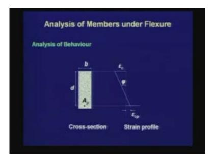
This sketch shows the definition of curvature which is equal to the gradient of the strain profile.
