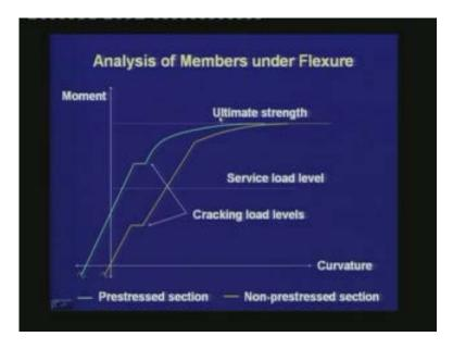
If we look at the two values of curvature from the two curves at a particular value of the moment, we see that the curvature in the prestressed concrete member is less than the curvature of the reinforced concrete member. Hence, prestressing reduces curvature at
