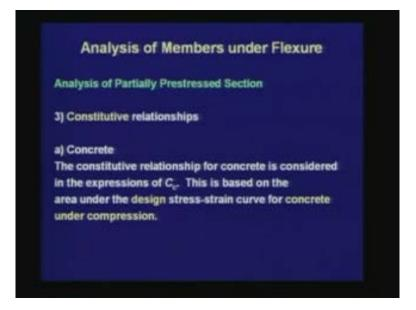
Next we move on to the constitutive relationships. A constitutive relationship relates the stress and strain in a material. For concrete, the constitutive relationship is considered in the expression of  $C_c$  which we had seen earlier. This is based on the design stress–strain curve for concrete under compression.
