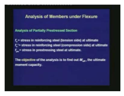
We also do not know the stresses in the steel at ultimate:  $f_s = stress$  in reinforcing steel for the tension side,  $f'_s = stress$  in reinforcing steel for the compression side,  $f_{pu} = stress$  in prestressing steel. With this set of known and unknown quantities, the objective of an analysis is to find out  $M_{uR}$ , the ultimate moment capacity. (Refer Slide Time: 23:40)
