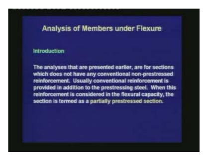
The analyses that are presented earlier are for sections which do not have any conventional non-prestressed reinforcement. Usually, conventional reinforcement is provided in addition to the prestressing steel. When this reinforcement is considered in the flexural capacity, the section is termed as a partially prestressed section.
