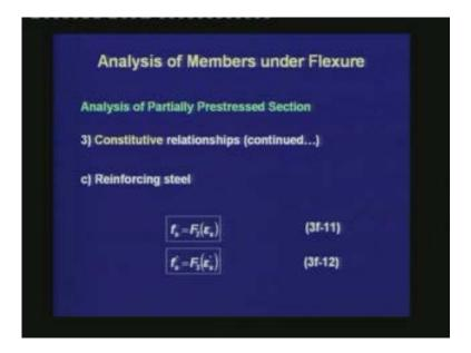
The third constitutive relationship is for the reinforcing steel of two layers. The equation for the bottom layer near the tension face is represented as  $f_s = F_2(\epsilon_s)$ . The equation for the steel near the compression face is equal to  $f_s^{\prime} = F_3(\epsilon_s^{\prime})$ .
