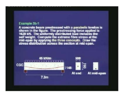
Next, we are solving a problem. A concrete beam prestressed with a parabolic tendon is shown in the figure. The prestressing force applied is 1620 kN. The uniformly distributed load of 45 kN/m includes the self-weight. Compute the extreme fibre stress at the mid-span by applying the three concepts. Draw the stress distribution across the section at mid-span.
