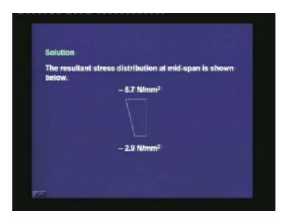
The resultant stress distribution at mid-span is shown. The compressive stress at the top is  $-5.7 \text{ N/mm}^2$  and the compressive stress at the bottom is  $-2.9 \text{ N/mm}^2$ . We see that this member is subjected to compression throughout the depth of the section under the service loads.
