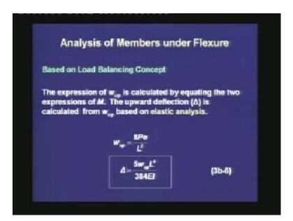
The upward deflection  $\Delta$  is calculated from  $w_{up}$  based on elastic analysis. The expression is  $\Delta = 5w_{up}L^4/384EI$ . This we have got from the analysis of a beam under uniformly distributed load. Here, the uniformly distributed load is upwards which is represented as  $w_{up}$ . Hence, the deflection is also upwards which is known as camber due to prestressing. The camber is given as  $5w_{up}L^4/384EI$ . Here, E is the modulus of concrete and I is the moment of inertia.
