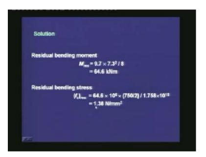
The residual bending moment is equal to  $M_{res} = w_{res} L^2/8 = 64.6$  kNm. The residual bending stress, which is the stress due to the residual bending moment, is equal to My/I. Here once we substitute the values of the variables, we get a value of 1.38 N/mm<sup>2</sup>. Hence, this is the bending stress which is created by the residual bending moment.
