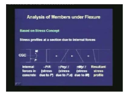
For this beam, the stress diagrams at a particular section are as follows. At any particular section, we are identifying the internal forces that are acting in the concrete. First is the prestressing force which is being transferred by the tendon to the concrete and it is compressive. The second is the moment which is acting due to the weight of the beam. Remember that at service loads, M includes the moment due to self-weight and that due to the service loads.
