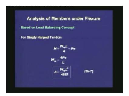
There are two expressions of the moment: one based on the central point load where  $M = W_{up} L/4$  and the second is, M = Pe. Once we equate these two expressions of M, we get an expression of  $W_{up}$  which is equal to 4Pe/L. We can calculate the upward deflection or the camber from the structural analysis formula.  $\Delta = W_{up}L^3/48EI$  where, E is the modulus of concrete.
