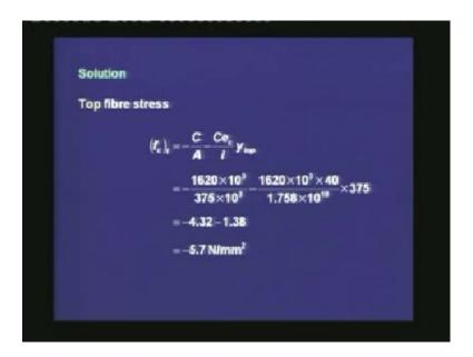
If we calculate the top fibre stress, by the expression  $(f_c)_t = -C/A - Ce_c y_{top}/I$ . Here we are selecting minus for the second term because the compression creates compressive stress at the top. Once we substitute the values of the quantities, we get the same result as from the stress concept, which is  $-5.7 \text{ N/mm}^2$ .
