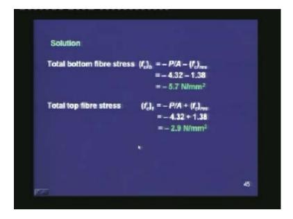
The total bottom fibre stress  $(f_c)_b = -P/A - (f_c)_{res}$  (minus because in the bottom we have a compressive stress), and once we substitute the values, we get the same value as that by the stress concept, which is  $-5.7 \text{ N/mm}^2$ . The top fibre stress is given as  $-P/A + (f_c)_{res} = -2.9 \text{ N/mm}^2$ .
