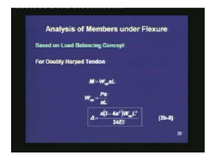
If we equate the two expressions of M,  $M = W_{up}aL$  which is derived from the moment diagram, and M = Pe. Then, we get an expression of  $W_{up}$  which is equal to Pe/aL. From structural analysis, we can find out the upward deflection  $\Delta = a(3 - 4a^2) W_{up} L^3 / 24EI$ .
