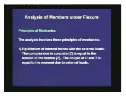
We also use the principles of mechanics. There are three principles of mechanics involved in the analysis. First is the equilibrium of internal forces with the external loads. The compression in concrete which will be represented as C, is equal to the tension in the tendon which will be represented as T. The second is, the couple of C and T is equal to the moment due to the external loads. This is the moment equilibrium equation.
