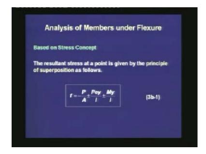
Once we have identified the stress components due to the forces in the concrete which are P and M, we can write an expression of the stress in the concrete for any depth in the section, and at any location in the beam. This expression is equal to  $-P/A \pm Pey/I \pm My/I$ . We shall use this expression frequently to check the stresses in concrete under service loads.
