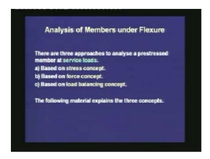
We know that there are three approaches to analyse a prestressed concrete member at service loads. First is based on the stress concept. Second is based on the force concept, and third is based on the load balancing concept. The following material explains the three concepts.
