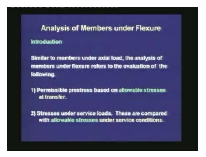
Last time, we studied the analysis of members under axial load. Similar, to members under axial load, the analysis of members under flexure refers to the evaluation of the following. First is the permissible prestress based on allowable stresses at transfer; second are the stresses under service loads. These are compared with allowable stresses under service conditions.
