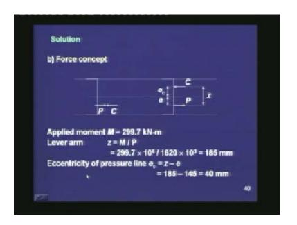
The same calculations, we are doing based on the force concept. Here the applied moment is equal to 299.7 kNm. Hence, the lever arm z is given by M / P which is  $299.7 \times 10^6$  (in Nmm) /  $1620 \times 10^3$  (in N) = 185 mm. At the center, the deviation of the compression from the CGS is equal to 185 mm, and that is the lever arm generated when the external load is applied on the member.
