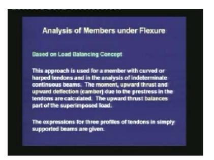
This is a very unique concept for prestressed concrete members. This approach is used for a member with curved or harped tendons, and in the analysis of indeterminate continuous beams. The moment, upward thrust and upward deflection are calculated. The upward thrust balances part of the superimposed load. This approach is thus termed as the load balancing concept.
