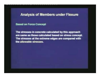
If we calculate the stresses based on this approach then they will come out to be same as those calculated based on the stress concept. The final results of the stresses based on the stress concept or based on the force concept, are the same. Both the concepts will give the same values of the stresses in the concrete. The stresses at the extreme edges are compared with the allowable stresses under service conditions.
