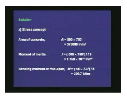
First we are solving the problem by the stress concept. We are finding out the geometric properties. The area of the concrete is  $500 \times 750 = 375,000 \text{ mm}^2$ . The moment of inertia is given as the 500 (breadth) ×  $750^3$  (depth) /  $12 = 1.758 \times 10^{10} \text{ mm}^4$ . The bending moment at mid-span due to the external loads is given as  $M = 45 \times 7.3^2 / 8 = 299.7 \text{ kNm}$ .
