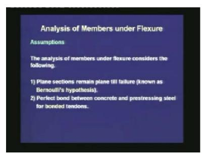
The assumptions of analysis of members under flexure, considers the following. First, plane sections remain plane till failure. This is the basic assumption of beams under flexure and this is known as the Bernoulli's hypothesis. Based on this, we draw the strain diagram, which is linear across the depth of a section at any instance of the complete load versus deformation behaviour. That means, we consider that the assumption is valid till the failure of the member.
