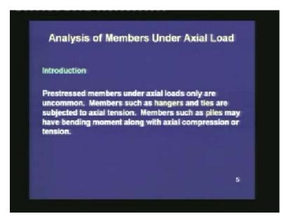
Prestressed concrete members only under axial loads, are uncommon. Members such as hangers and ties are subjected to axial tension. Members such as piles may have bending moment along with axial compression or tension.
