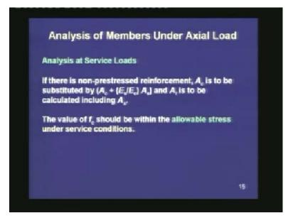
If there is non-prestressed reinforcement, then the area  $A_c$  is to be substituted by  $A_c$  plus the modular ratio times  $A_s$ , and the transformed area  $A_t$  is to be calculated including  $A_s$ . That is, the way we have included  $A_s$  in the previous expression, similarly, we shall include  $A_s$  in this expression as well.
