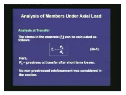
The stress in the concrete can be calculated as follows. The stress is given as the ratio of the prestress at transfer after short-term losses divided by the area of the concrete. In this expression, we have not considered any non-prestressed reinforcement. Just note that we are considering a negative sign for a compressive stress under the prestressing force.
