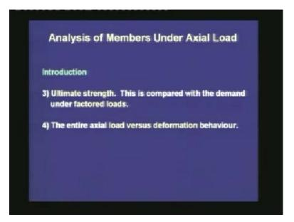
Third, we shall study the ultimate strength. This is compared with the demand under the factored loads. That means, in a limit state design, we compare the ultimate strength with the demand under ultimate loads, which are the load factors times the characteristic loads. Finally, we shall study the entire axial load versus deformation behavior to understand the full property of the prestressed concrete member. First, we are studying the analysis at transfer.
