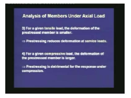
The third statement is, for a given tensile load, the deformation of the prestressed concrete member is smaller.
