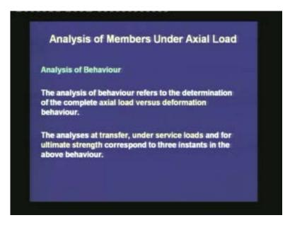
The analysis of behavior refers to the determination of the complete axial load versus deformation behavior. The analyses at transfer, under service loads and for ultimate strength correspond to three instants in the above behavior. Whatever we have studied till now are just three points in the complete load versus deformation behavior. The load versus deformation behavior is an entire curve, which shows how the member will behave, when we are gradually increasing the externally applied load.
