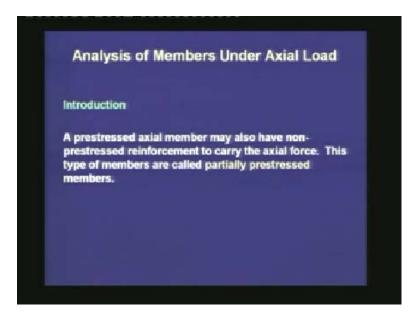
A prestressed axial member may also have non-prestressed reinforcement to carry the axial force. This type of members is called partially prestressed members. We shall also come back to partially prestressed members for flexure. This type of members is somewhere in between the reinforced concrete members and fully prestressed members. The partially prestressed members have both prestressing tendons and non-prestressed reinforcement to carry the forces.
