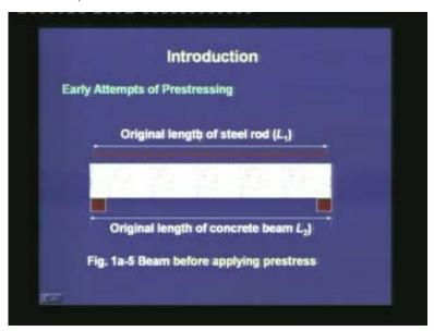
Let us try to understand this by a simple sketch. In this beam, the original length of the steel rod was  $L_1$ . It has been tensioned to a length which is equal to the original length of the concrete beam, that is  $L_2$ . This is the state of the beam before applying prestress.
