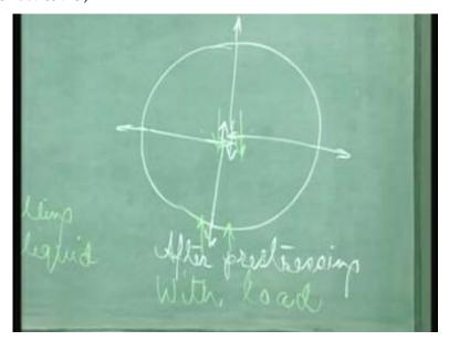
The second example is the cycle spokes. Due to the tensioning of the spokes, each of the spokes is under tension. When the rider rides on the cycle, the weight creates some compression in the spoke; but since there was an original tension and this tension is
