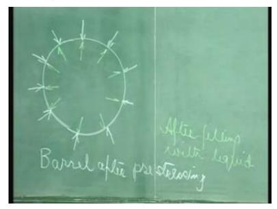
When the barrel is first prestressed, the prestressing causes a hoop compression throughout the barrel. Next, we are filling this barrel with liquid; this liquid creates a hoop tension. The hoop tension that is created by the liquid is counteracted by the hoop compression that is generated due to the prestressing.
