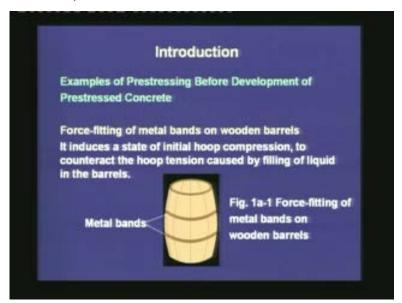
The first one is the force-fitting of metal bands on wooden barrels. These types of barrels were used to transport liquid and oil, and types of grains. Now, what the prestressing does is that, the metal bands create a hoop compression around the barrel. When this barrel is filled with liquid, the liquid tries to push out; it creates a hoop tension. The hoop
