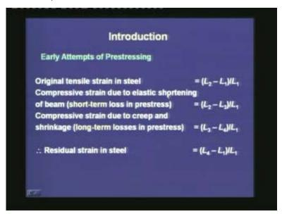
For the example that we have shown before, the original tensile deformation in the steel was  $L_2$  minus  $L_1$ , where  $L_2$  was the original length of the beam and  $L_1$  was the original length of the steel rod. That means, when the rod was tensioned, the strain in the steel was given as  $L_2$  minus  $L_1$  divided by  $L_1$ .
