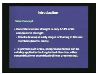
Why do we need prestressing for concrete? The main reason is the concrete's tensile strength is only 8 to 14 percent of its compressive strength; this is the weak point of concrete. For flexural members, cracks develop at early stages of loading. Examples of flexural members are beams and slabs. If we gradually load the structure, we shall observe that cracks are being generated in the flexural members.
