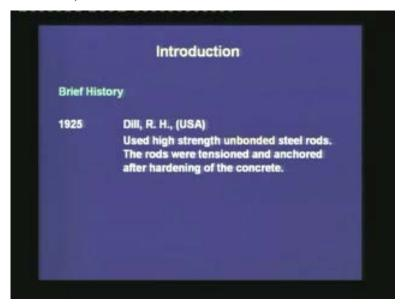
In 1925, Dill of USA used high strength unbonded steel rods. The concept of unbonded means, that there was no bond or, there was no physical stress transfer between the steel and the concrete at the interface. The transfer of stress was only at the ends. The reason of using an unbonded steel rod was that the rods could be tensioned and anchored after hardening of the concrete, and they could be again tightened so as to counteract the drop in the prestress.
