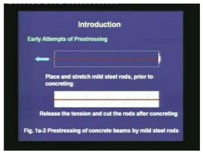
In the earlier days, the way the prestressing was done was that, initially a rod used to be pulled with an anchor at one end and then in the mould, the concrete used to be placed. Once the concrete has hardened, the tension used to be released in the tendon and then
