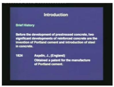
Before I start the development of prestressed concrete, let us know two significant developments of reinforced concrete itself. The two major breakthroughs in the development of reinforced concrete are: first, the invention of Portland cement and second is the introduction of steel in concrete; that means, the whole concept of reinforcing the concrete by steel was a very innovative concept at that time.
