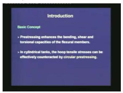
The prestressing enhances not only the bending capacity, but it also enhances the shear and the torsional capacities of the flexural members. In the subsequent modules of this course, we shall see that both the shear capacity and the torsional capacity are enhanced due to the pre-compression that is introduced by the prestressing.
