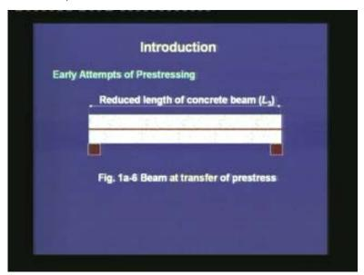
When the rod is cut, since the steel is applying compression in the concrete, the concrete will tend to compress; this is called the phenomenon of elastic shortening. After the elastic shortening, the length of the beam reduces to  $L_3$  which is lower than the initial
