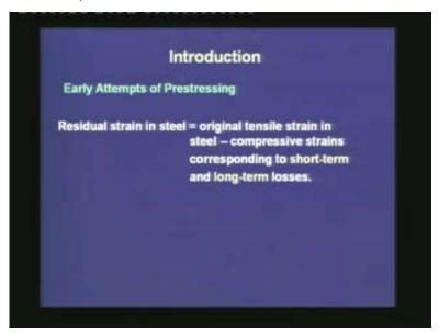
We have to calculate what the residual strain in the steel is, because it is the residual strain which will have the residual prestress. The residual strain can be calculated as the original tensile strain in steel minus the compressive strains corresponding to short-term and long-term losses. In this expression, we shall consider the tensile strain to be positive and the compressive strains to be negative; that is why we have placed a subtraction for the compressive strains.
