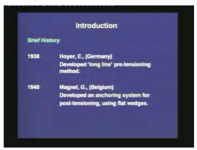
In 1938, Hoyer of Germany developed the long-line pre-tensioning method. This method can be compared with the assembly line method in the manufacture of cars. That is, under one industrial shed and in just one line, several prestressed members were being produced. This technique was used to produce pre-tensioned transmission poles for electric lines.
