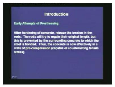
What happens is after the hardening of concrete and when the tension is released from the rods, the rods will try to regain their original length, but this is prevented by the surrounding concrete to which the steel is bonded. Thus, the concrete gets effectively under a state of pre-compression which is capable of counteracting the tensile stresses.
