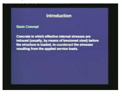
Concrete in which effective internal stresses are induced (usually, by means of tensioned steel) before the structure is loaded, to counteract the stresses resulting from the applied service loads. Here also the concept is similar. That is, after prestressing when the structure is subjected to the external loads, the stresses due to prestressing counteracts the stresses due to the external loads.
