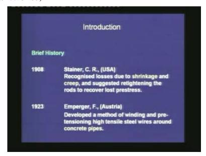
In 1908, Stainer of USA recognized the losses due to shrinkage and creep. This was a major breakthrough to understand the problem of reduction of the effective prestress with
