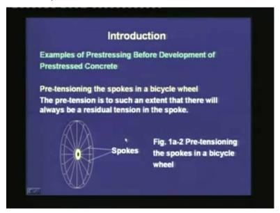
The second example is the pre-tensioning of the spokes in a bicycle wheel. Here you can see that in a bicycle wheel, each one of these spokes is pulled and tightened. This pre-tension is to such an extent that there will always be a residual tension in the spoke. Let me explain these two examples on the black board.
