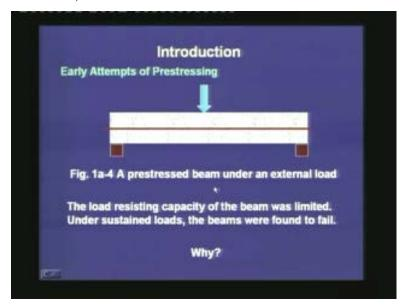
It was observed that, this type of simple beams which were prestressed initially may have a good flexural capacity. But with time, it was found that the flexural resisting capacity got limited and if the load is kept sustained, it was observed that sometimes the beams tend to fail. The question that comes to our mind is why does it happen so? Initially it is found to be effective, but with time it is found that the effect of prestressing is getting reduced. Why is this so?
